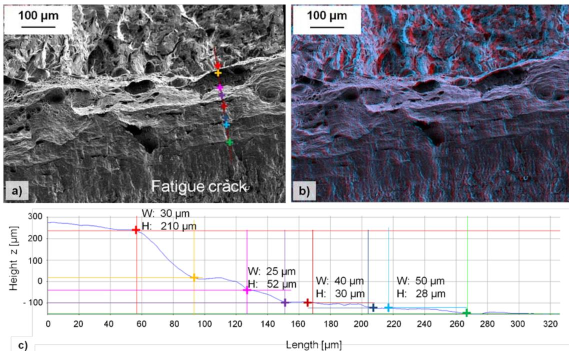
Figure 2: Multiple stretch zones in a high strength construction steel. (a) 2D SEM micrograph using SE contrast. (b) 3D anaglyph image. (c) Corresponding height profile along the measuring line indicated in (a) with determined values for SZW and SZH.
