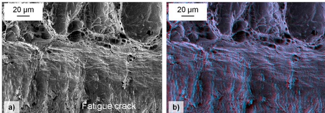
Figure 4: Stretch zone on a fracture surface of 10CrMo9-10. (SENB, tested at RT). (a) 2D SEM micrograph using secondary electron contrast. (b) 3D anaglyph image.
