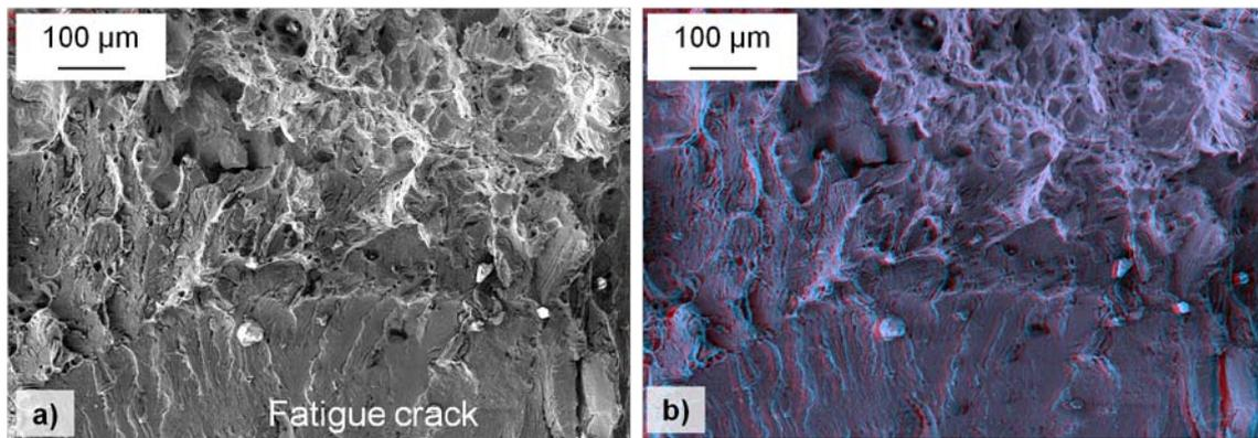
Figure 3: Multiple stretch zones in a high alloyed cast TRIP steel (16%Cr 6%Mn 6%Ni) SENB 10 mm deformed at 20°C. (a) 2D SEM micrograph using SE contrast. (b) 3D anaglyph image.
