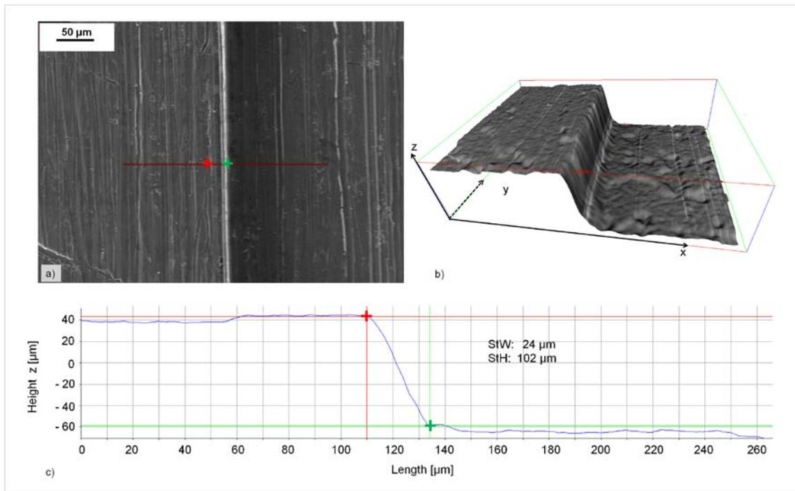
Figure 1: Reference specimen – aluminium cube with defined step height of 100 μm manufactured by milling. (a) 2D SEM micrograph. (b) 3D digital object micograph after reconstruction. (c) Height profile with measurement of step width (StW) and step height (StH).
