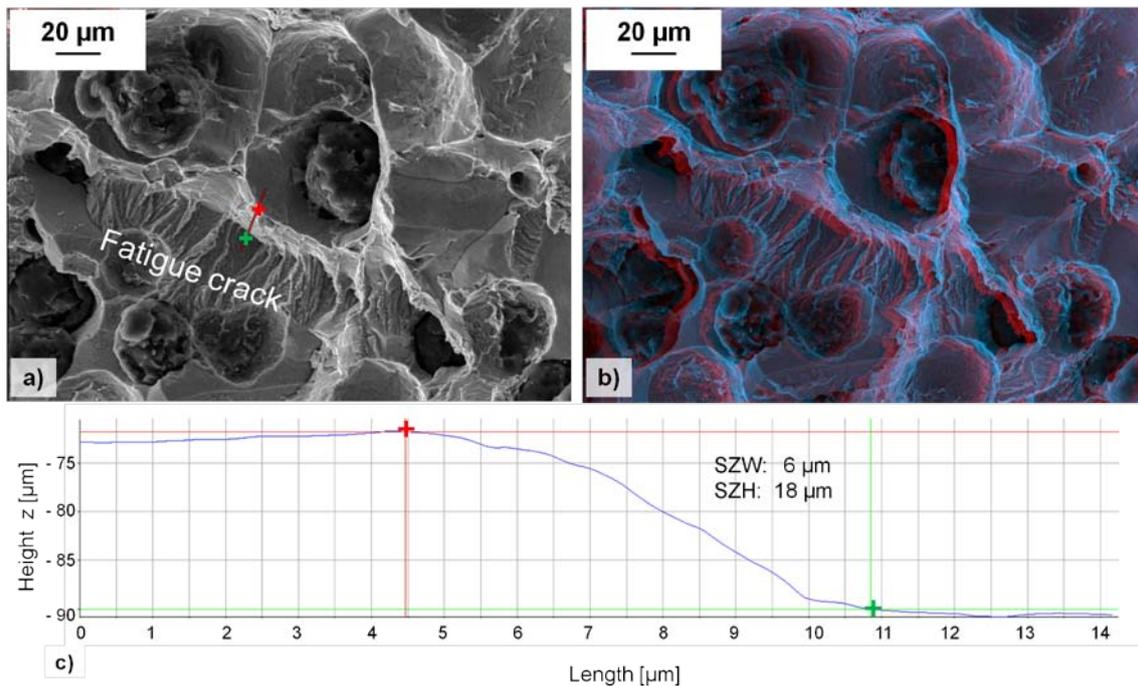
Figure 6: Stretch zone in a ductile cast iron. (a) 2D SEM micrograph taken in SE contrast. (b) 3D anaglyph image. (c) Height profile along the measuring line indicated in (a) with the measurement of the stretch zone width (SZW) and stretch zone height (SZH).
