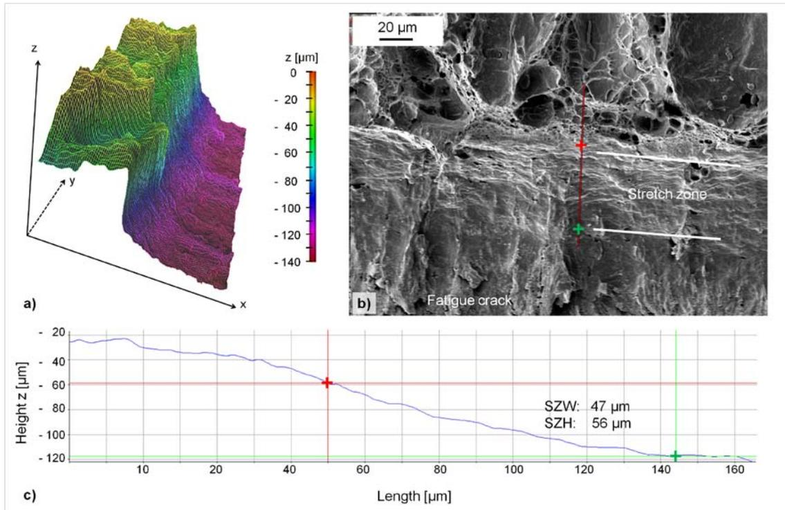
Figure 5: Measurement of the stretch zone width (SZW) and stretch zone height (SZH). (a) 3D reconstruction of the stretch zone obtained from two stereographic images taken at  $2.0^\circ$  tilt angle of the primary electron beam. (b) SEM micrograph with indicated measuring line and measuring points. (c) Corresponding height profile with determined values for SZW and SZH.
