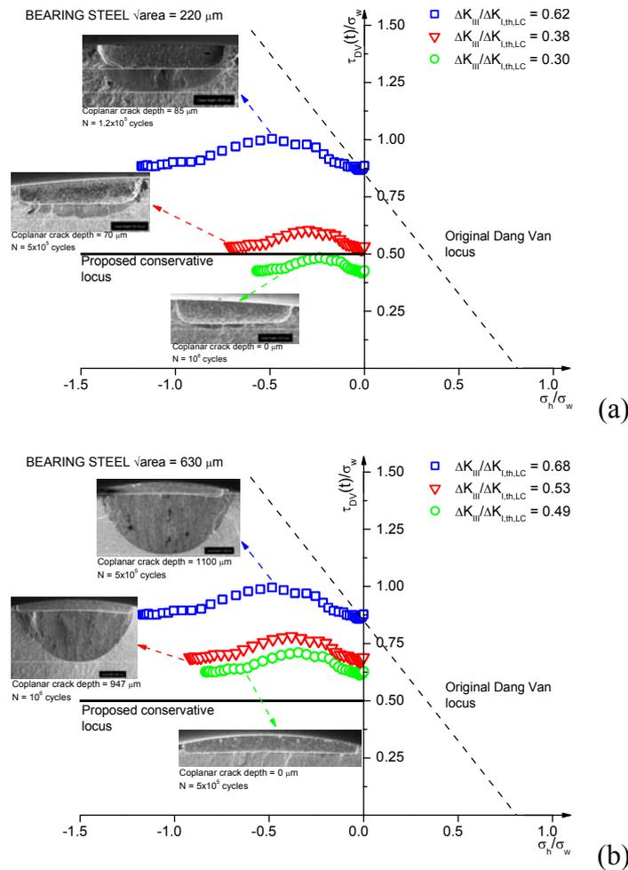
Figure 6. Application of Dang Van's criterion. Bearing steel- Load Path 1. a) defect size  $\sqrt{\text{area}} = 220 \mu\text{m}$ , b) defect size  $\sqrt{\text{area}} = 630 \mu\text{m}$ .
