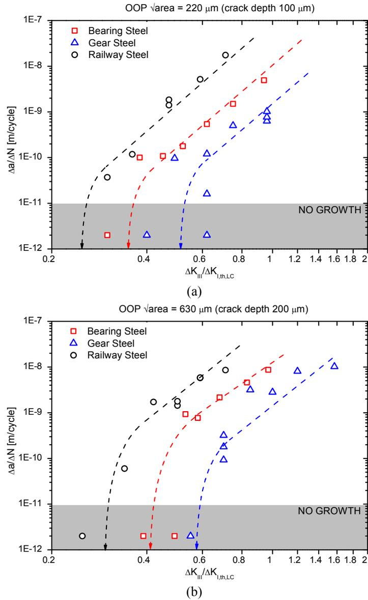
Figure 5. Coplanar crack growth rate under out-of-phase fatigue tests. a) defect size  $\sqrt{\text{area}} = 220 \mu\text{m}$ , b) defect size  $\sqrt{\text{area}} = 630 \mu\text{m}$ .
