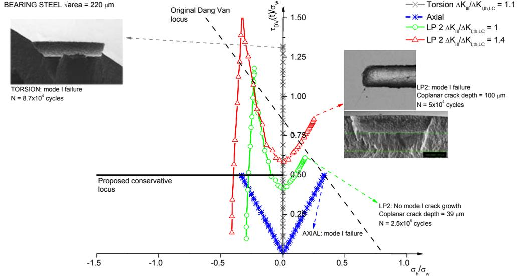
Figure 7. Application of Dang Van's Criterion. Bearing steel – Tension-compression, torsion and LP2. Defect size  $\sqrt{\text{area}} = 220 \mu\text{m}$ .
