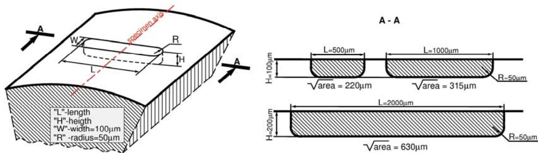
Figure 1. Micronotches adopted for fatigue tests.
