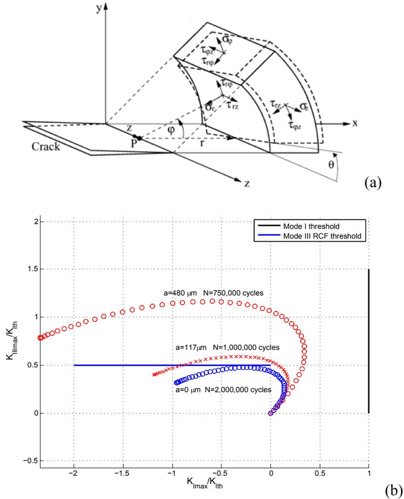
Figure 9. Analysis of OOP tests in terms of SIF's: a) cylindrical coordinate system along the crack; b)  $k_{I,max}$ - $k_{III,max}$  plots for the the out-of-phase tests onto the gear steel.
