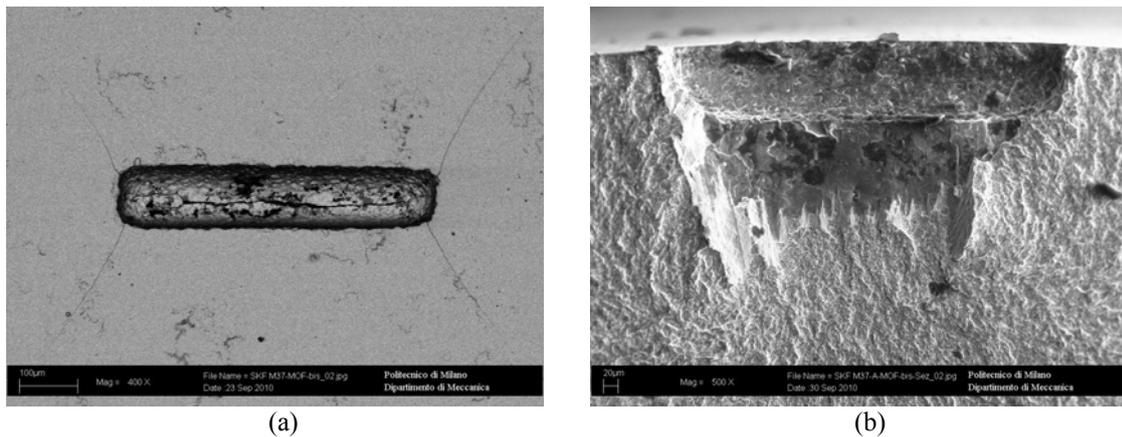
Figure 4. Fatigue test results onto the bearing steel under load path 2. (a) Mode I kinks, (b) Coplanar propagation
