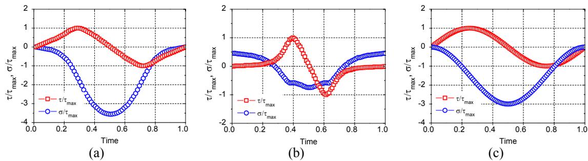
Figure 2. Load patterns. (a) Load Path 1 (LP1) – Bearing steel, (b) Load Path 2 (LP2) – Bearing steel, (c) Load Path 3 (LP3) – Gear steel and R7T steel.
