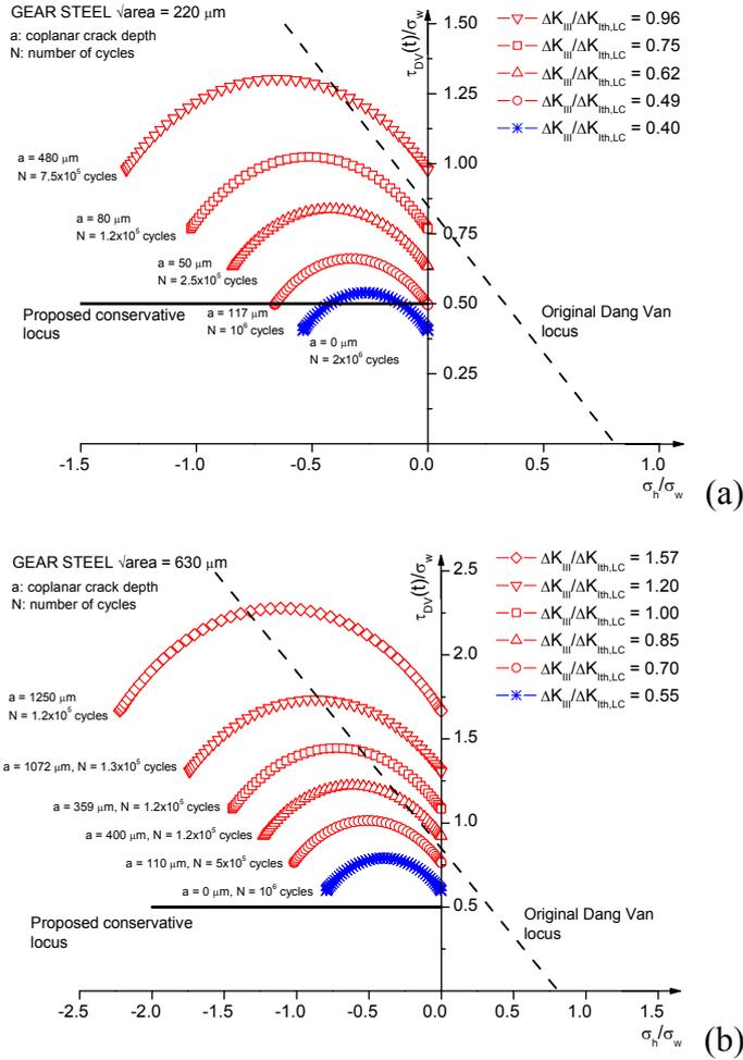
Figure 8. Application of Dang Van's Criterion. Gear steel – Load Path 3. a) Defect size  $\sqrt{\text{area}} = 220 \mu\text{m}$ , b) Defect size  $\sqrt{\text{area}} = 630 \mu\text{m}$ .
