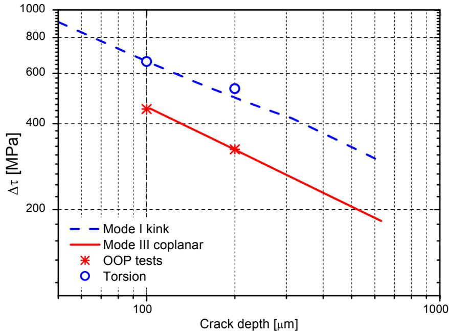
Figure 10. Dependence of fatigue limits on crack/defect depth for the gear steel.
