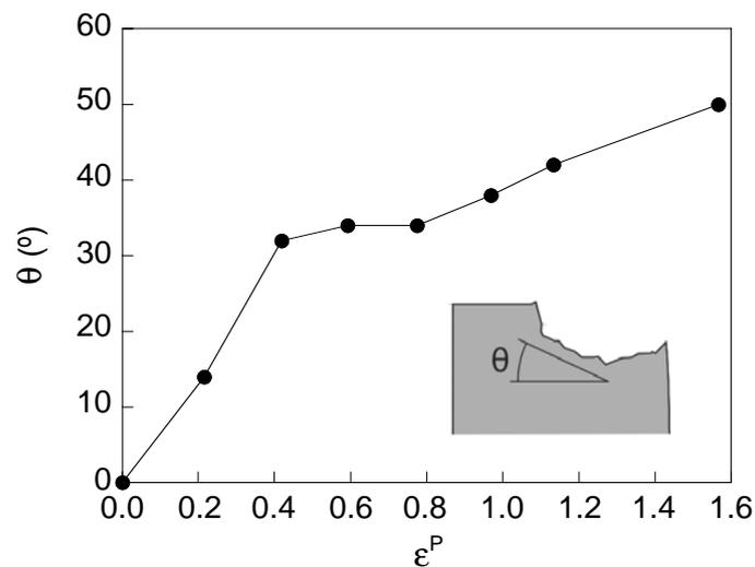
Figure 10. Crack deflection angle in the progressively drawn steels.
