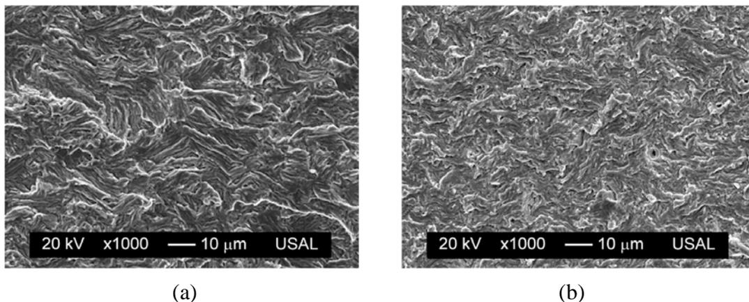
Figure 6. Fractographic analysis of the fatigue surface in the hot rolled bar E0 (a) and the prestressing steel wire E7 (b).
