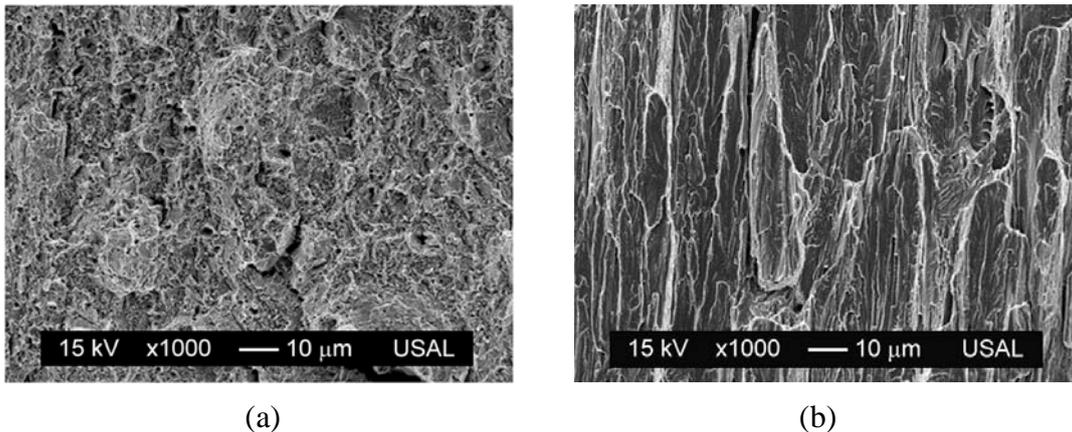
Figure 13. Horizontal (a) and vertical (b) fracture surface in the most heavily drawn steel (E7).
