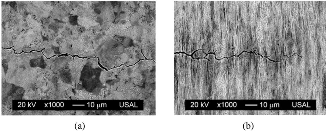
Figure 7. Fracto-metallographic analysis of the fatigue crack paths in the hot rolled bar E0 (a) and the prestressing steel wire E7 (b).
