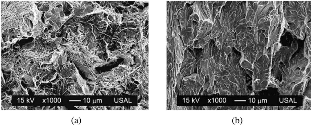
Figure 12. Horizontal (a) and vertical (b) fracture surface in a steel with an intermediate degree of drawing (E3).
