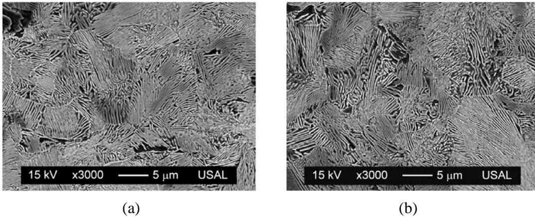
Figure 1. Scanning electron micrograph showing the microstructure of steel 0 (hot rolled bar that; not cold drawn at all): transverse section (a) and longitudinal section (b).
