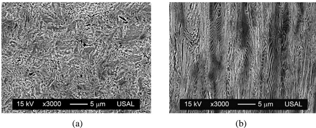
Figure 2. Scanning electron micrograph showing the microstructure of steel 7 (prestressing steel wire that has undergone seven steps of cold drawing): transverse section (a) and longitudinal section (b).
