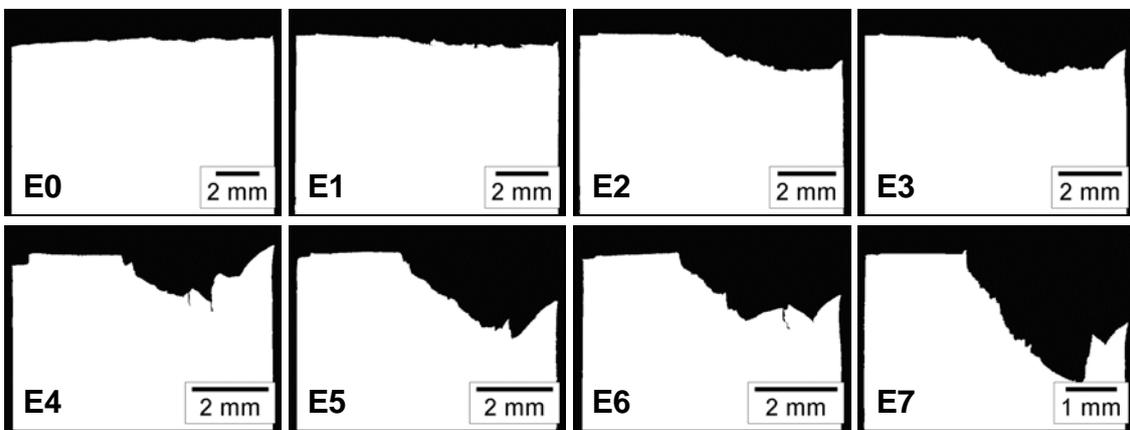
Figure 9. Fracture crack paths in the progressively drawn steels (from E0 to E7).
