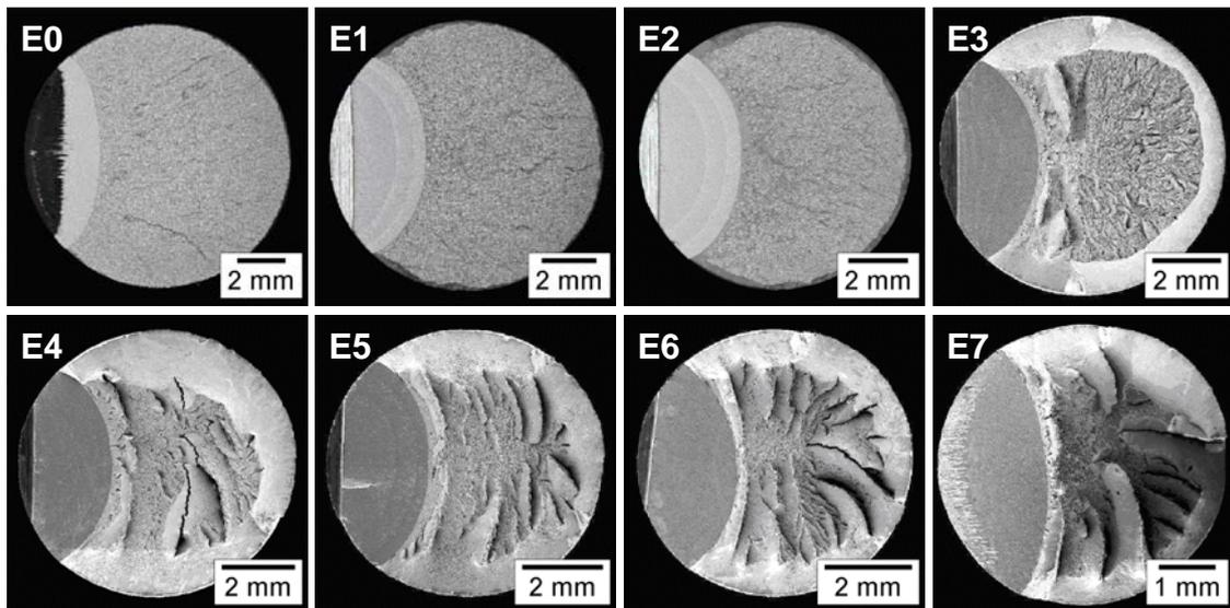
Figure 8. Fracture surface in the eight steels, from E0 to E7 (left to right and up to down). In all pictures fracture propagates from left to right.
