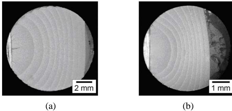
Figure 3. Fatigue crack front shapes for the hot rolled bar E0 (a) and the prestressing steel wire E7 (b).
