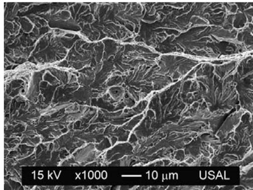
Figure 11. Main fracture surface by cleavage in the hot rolled steel (E0).
