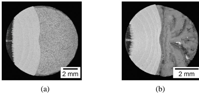
Figure 5. Fatigue crack front shapes in steels with an intermediate degree of cold drawing: E1 (a) and E6 (b).
