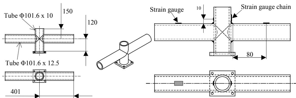
Figure 2. Geometry of the tested tubular welded joints.
