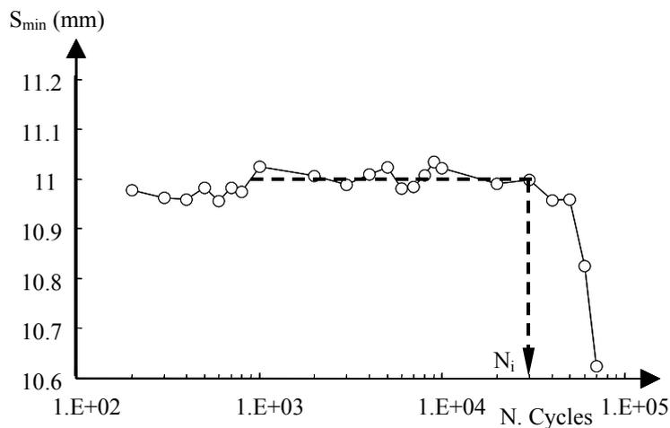
Figure 4. Typical stiffness drop measured during the experimental tests and engineering definition of fatigue life to crack initiation.
