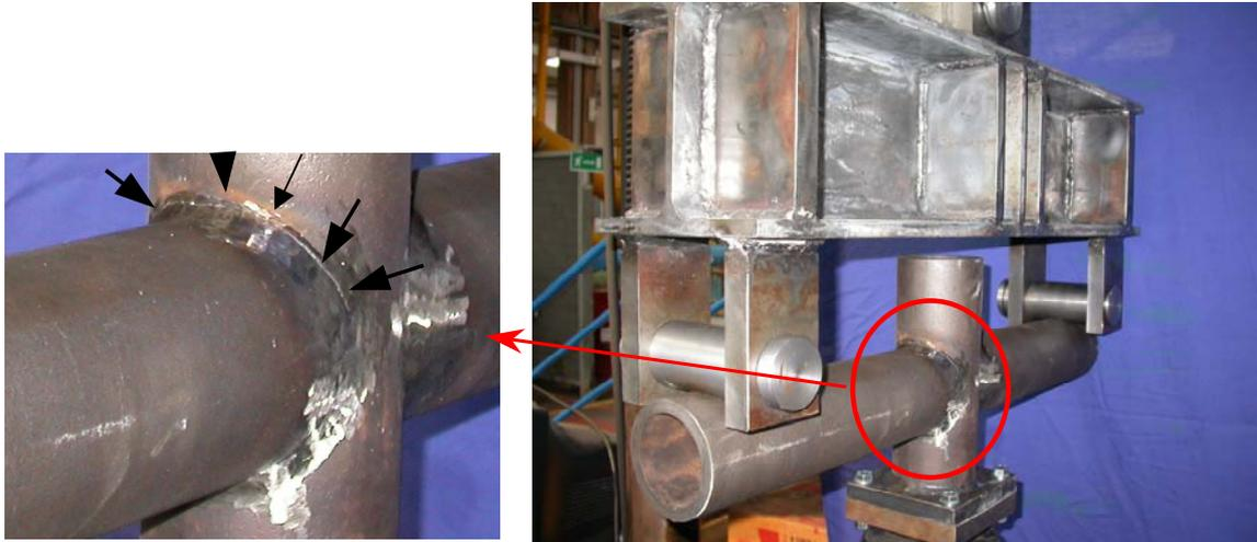
Figure 3. Adopted loading frame in the three point bending tests and typical crack propagation path observed after the fatigue test.
