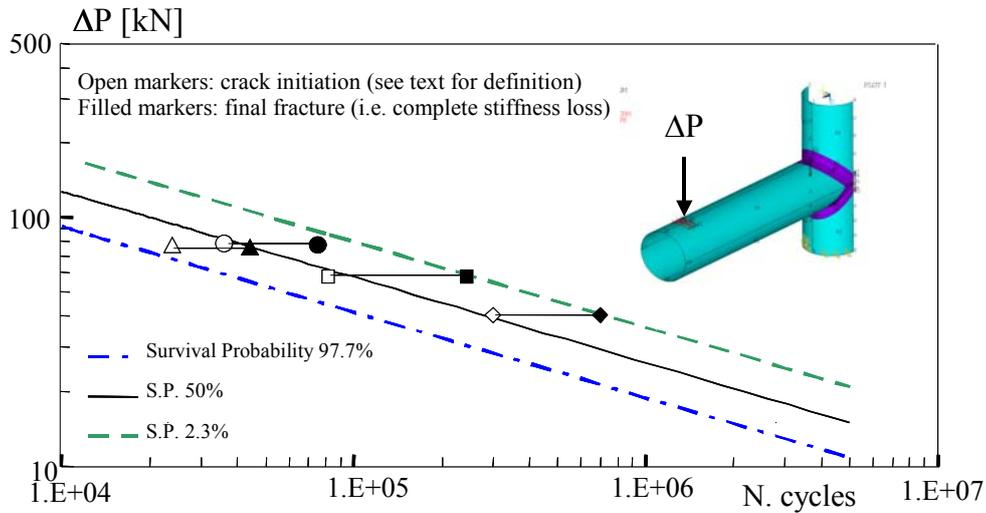
Figure 5. Fatigue test results of tubular welded joints. The scatter band is not a best fit of the experimental results.
