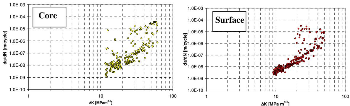
**Fig.2.** Paris curve for Steel A.
