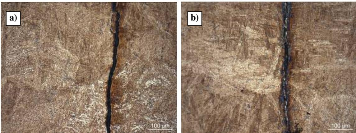
**Fig.7.** Crack path for steel B. Threshold zone (a) and stable propagation zone (b).
