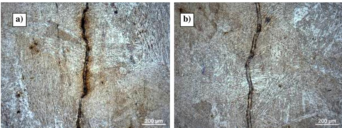
**Fig.6.** Crack path for steel A. Threshold zone (a) and stable propagation zone (b).
