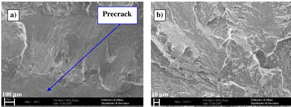
**Fig.4.** SEM images in the threshold zone (a) and in the stable crack propagation zone (b).
