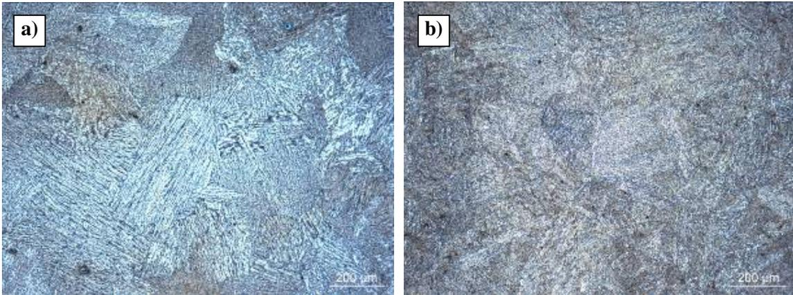
**Fig.5.** Microstructures observed in steel A at core (a) and in surface (b).
