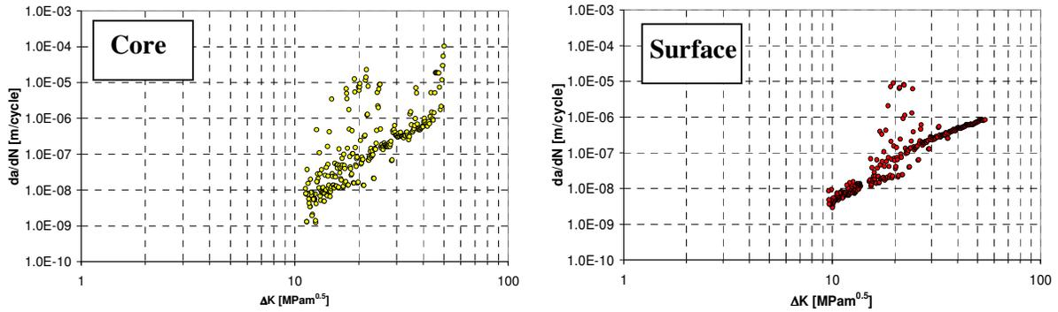
**Fig.3.** Paris curve for Steel B.
