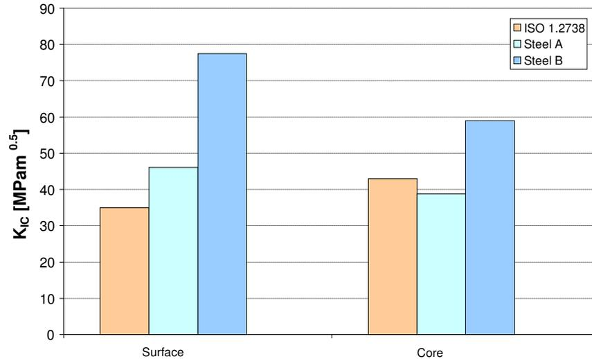
**Fig.1.** Toughness results for the investigated steels compared with ISO 1.2738.
