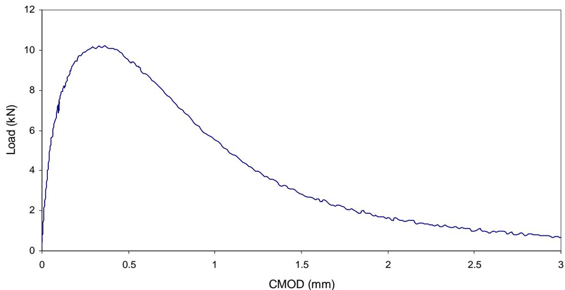
Figure 5 Load vs. CMOD for the untreated control specimen
