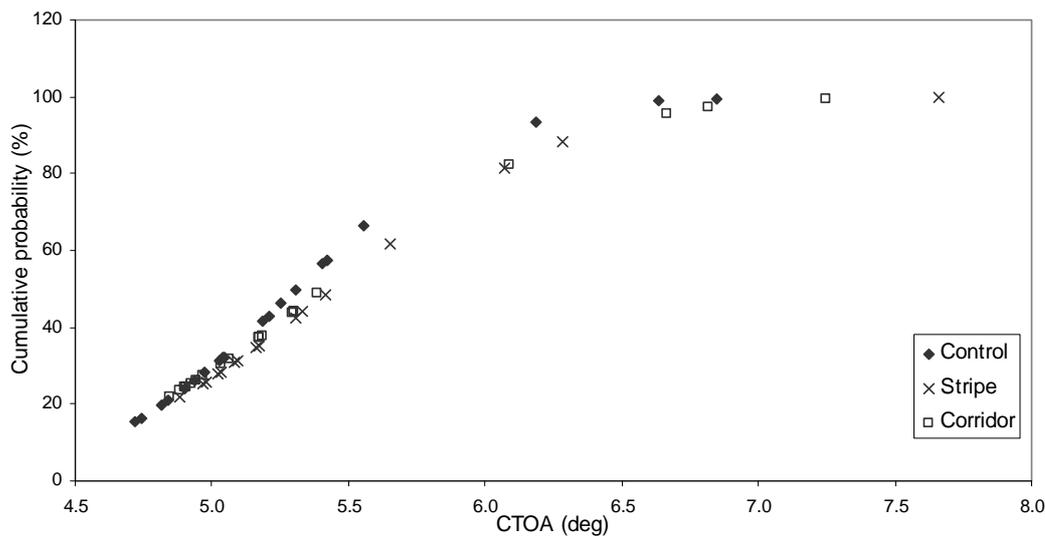
Figure 7 Cumulative probability curves for two burnished patterns and the control specimen, burnishing was at 2.12kN in both cases
