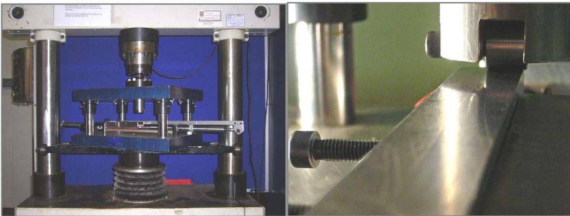
Figure 1 Burnishing apparatus left and closeup of the burnishing tool
