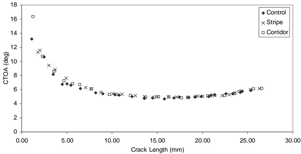
Figure 6 CTOA resistance for two burnished patterns and the control specimen, burnishing was at 2.12kN in both cases
