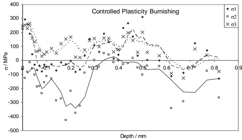
Figure 2 Principal residual stresses in CPB 2024-T351 measured with high energy XRD [1]
