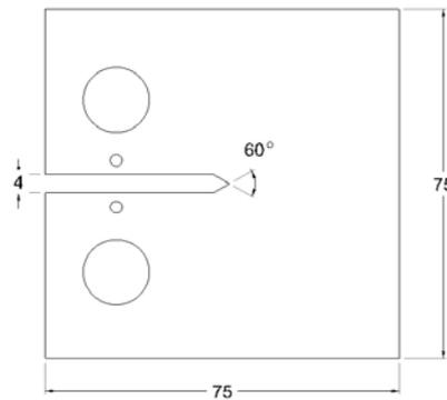
Figure 3 CT specimen dimensions, material was 5mm thick
