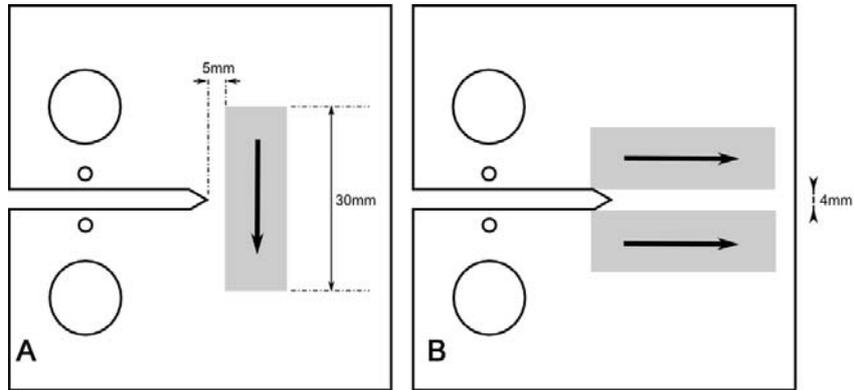
Figure 4 Burnishing patterns used, in both cases burnishing was repeated on the reverse side with feed in the same direction (A) Stripe and (B) Corridor
