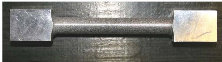
Figure 2: Prepared tensile specimen with speckle pattern on surface
