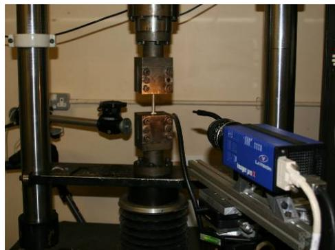
Figure 3: Tensile test experimental set-up with 2D DIC
