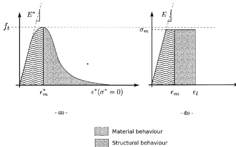
Figure 2: Principle of the equivalence for a uniaxial tensile behavior
