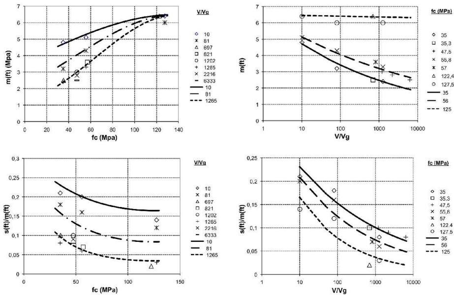
Figure 1: Tensile strength mean value/dispersion evolutions [1, 2, 3].
