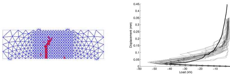
Figure 6: Typical crack patterns and crack opening (numerical -grey-, mean answer -circles- and experimental -bold-)
