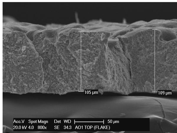
Figure 1. Cross-section of a monolayered coating
