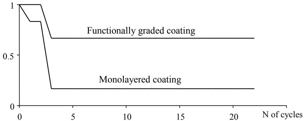
Figure 6. Ratio of the survived TBC to the total number of tested samples for functionally graded and monolayered coatings
