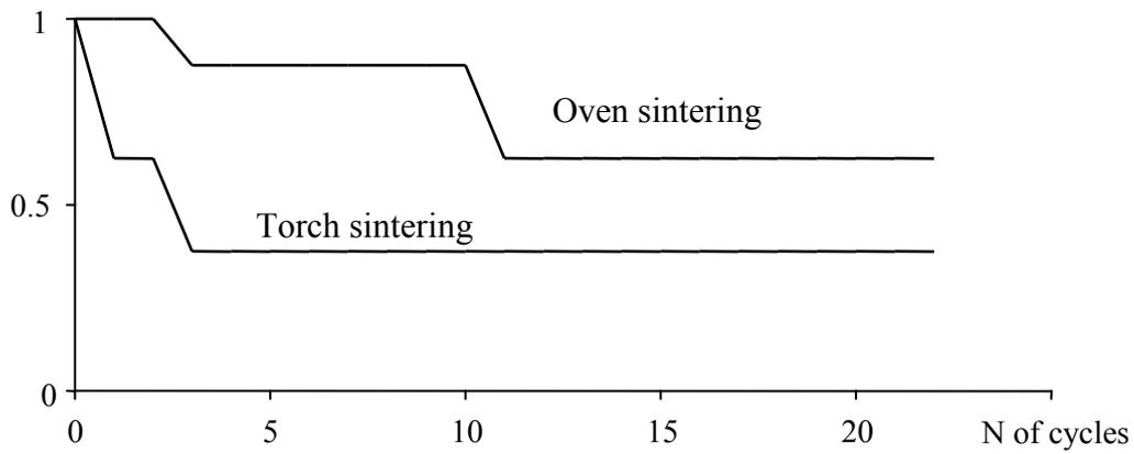
Figure 5. Ratio of the survived TBC to the total number of tested samples for oven and torch sintering
