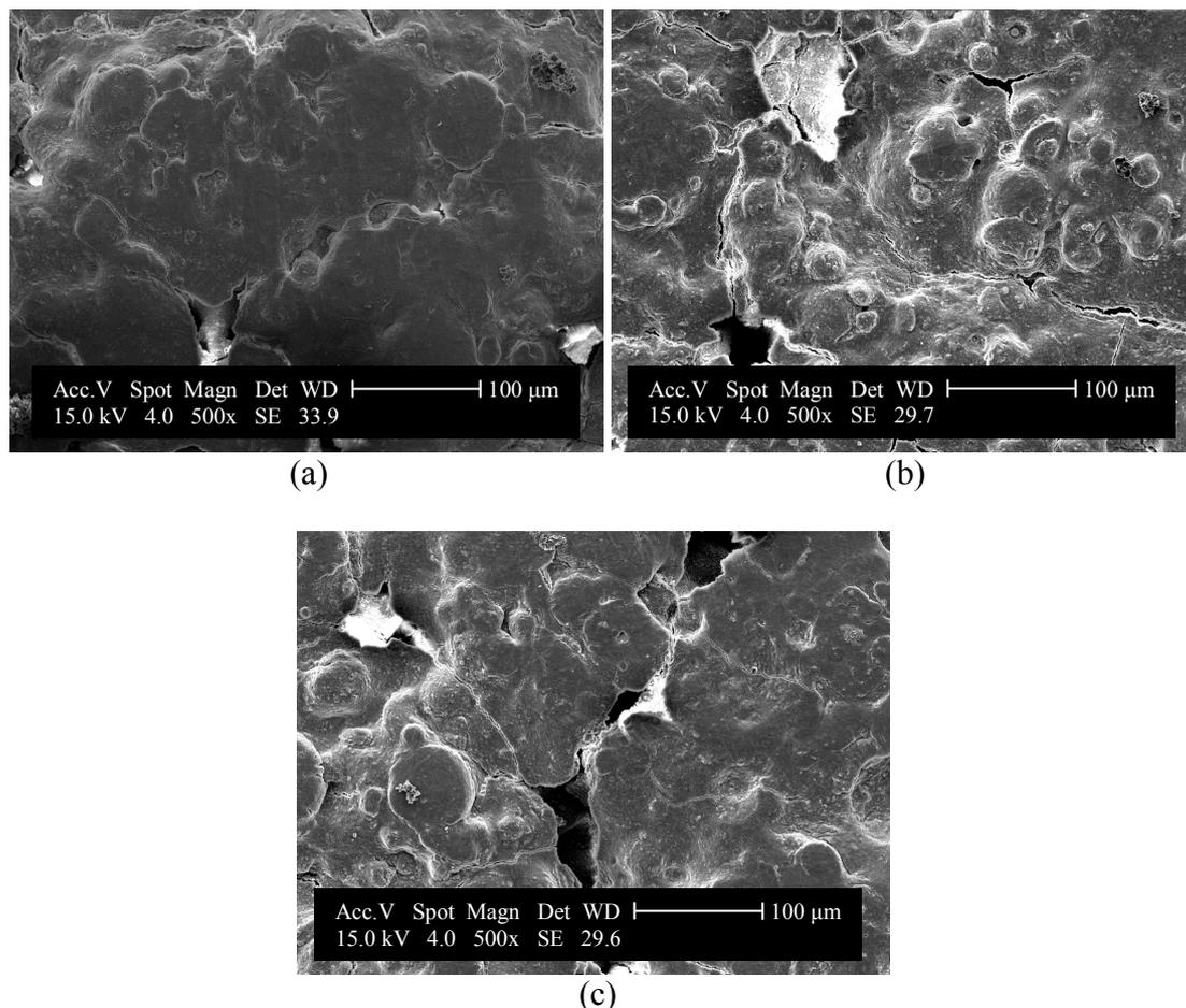
Figure 7. Microstructure of FG-TBC after fabrication (a), 10 thermal cycles (b) and 20 thermalcycles (c), magnitification – 500x.
