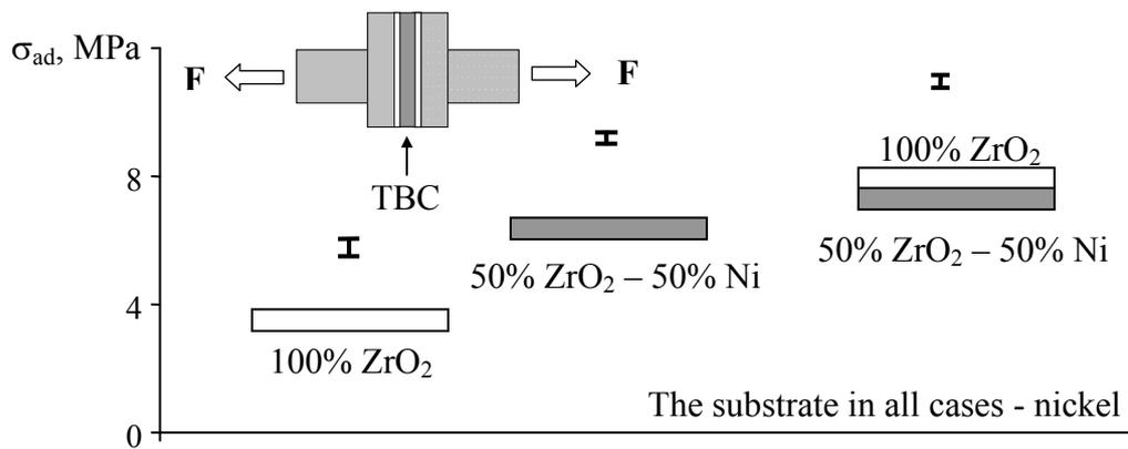
Figure 4. Adhesion strength range for various types of coatings
