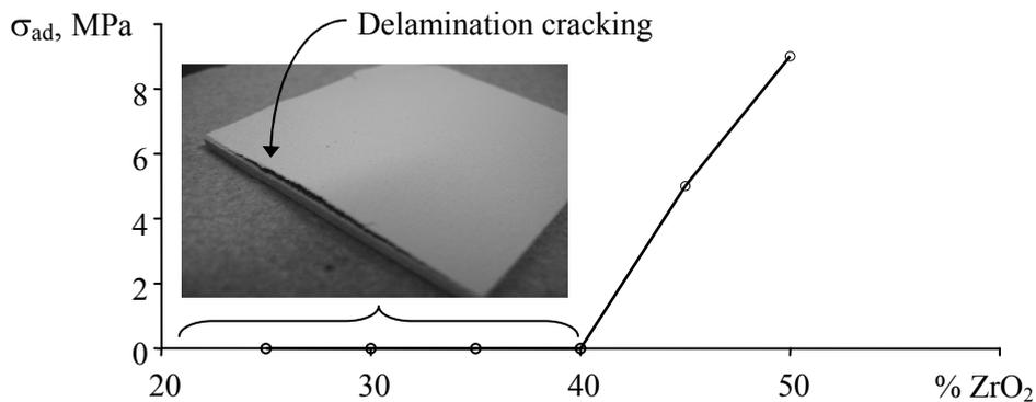
Figure 3. Adhesion strength of TBC versus zirconia contents
