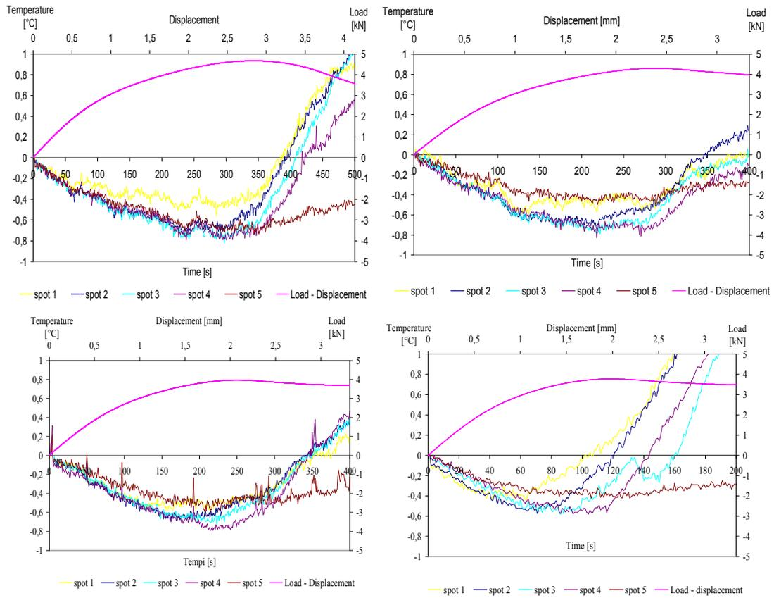
Figures 5 to 8. Thermal variation of the spots in the specimens with 4.5mm, 6.5mm, 8mm and 10mm hole diameter respectively.
