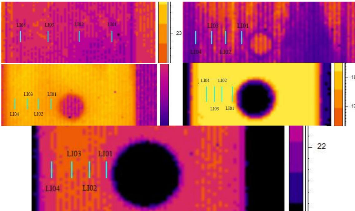
Figure 1. Thermal images with the spot position for the different hole diameters and the temperature scale (last image)
