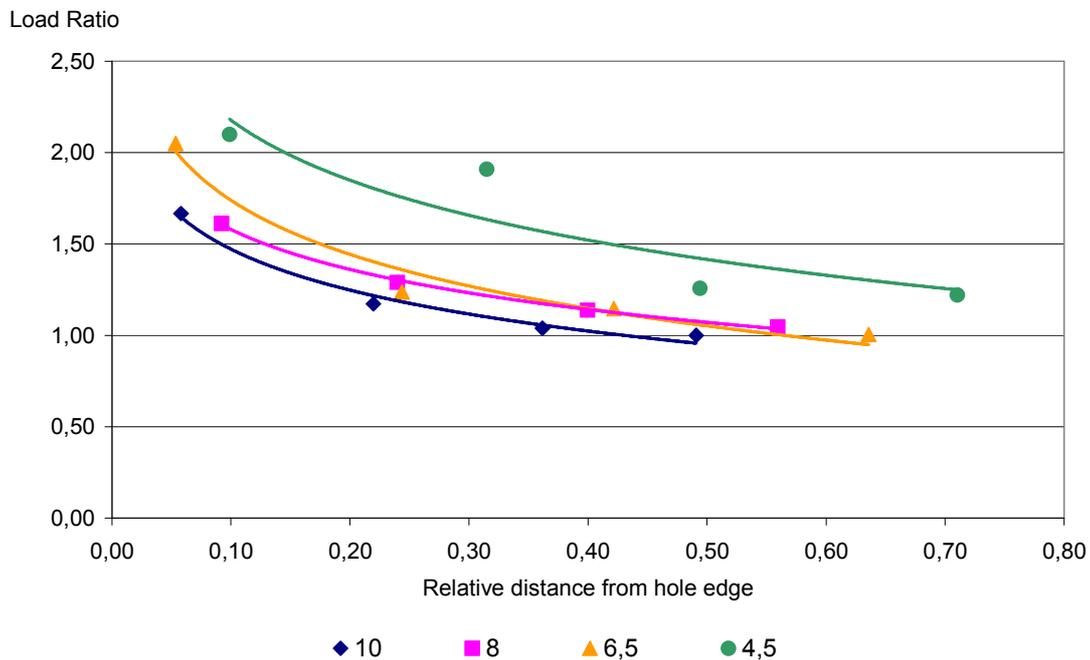
Figure 9. Load ratios for the specimens with 4.5mm, 6.5mm, 8mm and 10mm hole diameter respectively as a function of the relative distance.
