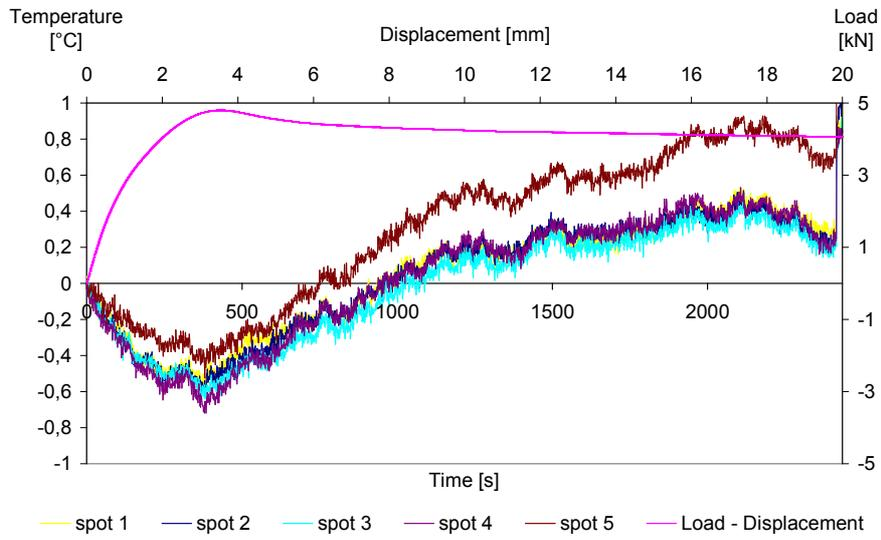
Figures 4. Thermal variation of the spots in the unnotched specimen.
