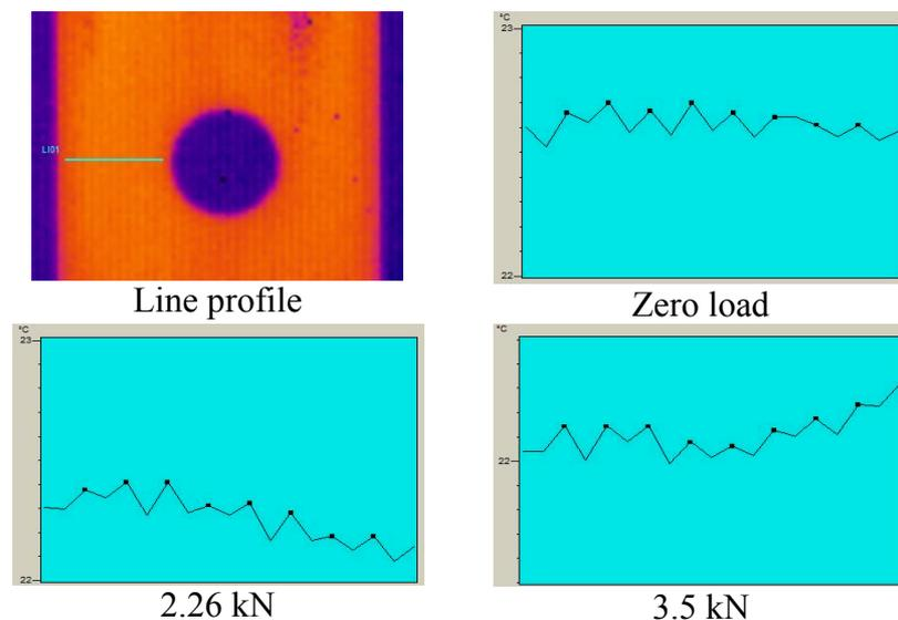
Figure 3. Sequence of temperatures along the cross line of the hole diameter.
