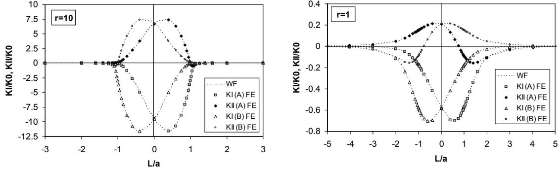
Fig. 3 SIF produced by the normal (compressive) force  $P_y$  travelling on the surface for two  $r$  ratios
