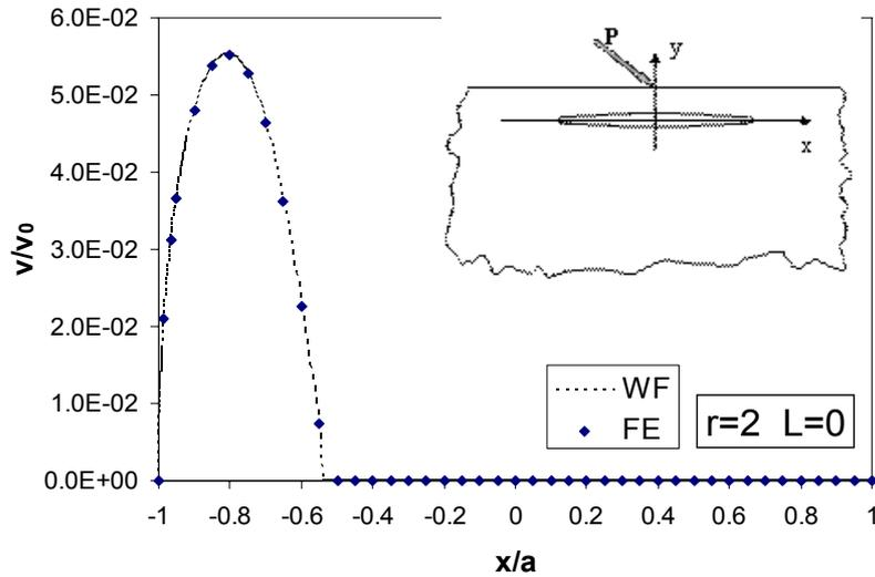
Fig. 5:  $v$  components of COD calculated by the GFs method and by the FE analysis. The  $v$  values are normalised by the following characteristic parameter  $v_0 = a\sigma_0/E$  ( $\sigma_0 = 2P/\pi a$ )
