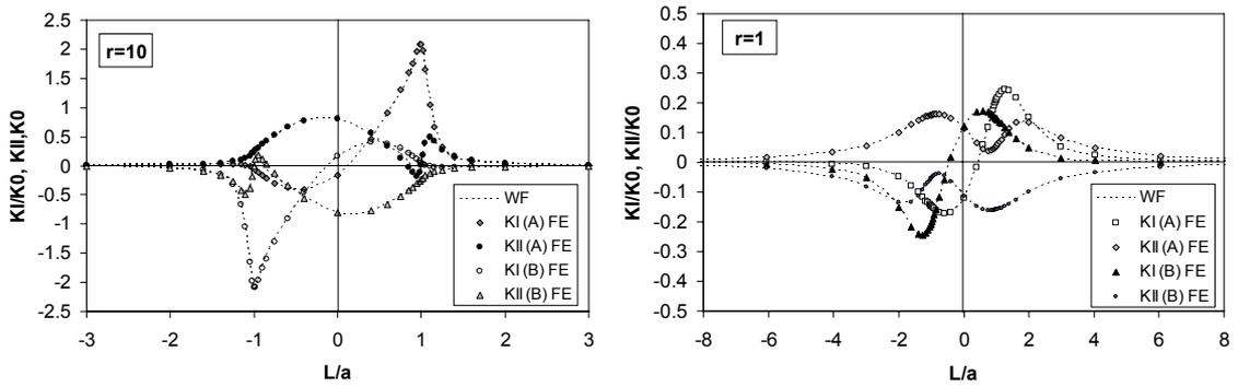
Fig. 4 SIF produced by the tangential force  $P_x$  travelling on the surface for two  $r$  ratios
