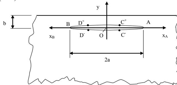
Fig.1 Subsurface crack parallel to the semiplane surface
