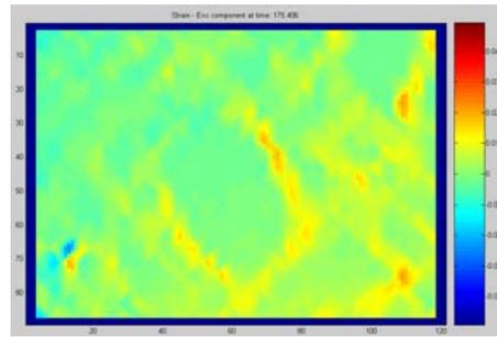
(b) Strains at fracture point
