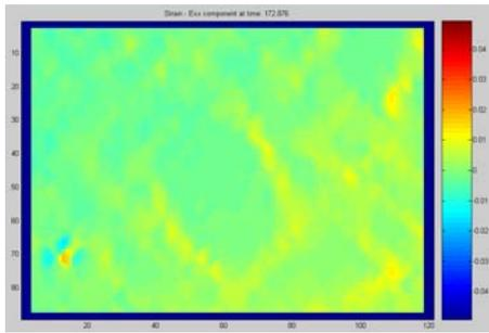
(a) Strains at cracks initiation
