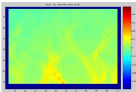
(a) Strains at cracks initiation
