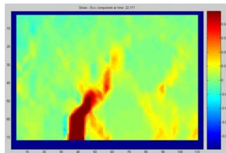
(b) Strains at fracture point
