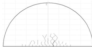
(b) Crack pattern at fracture point
