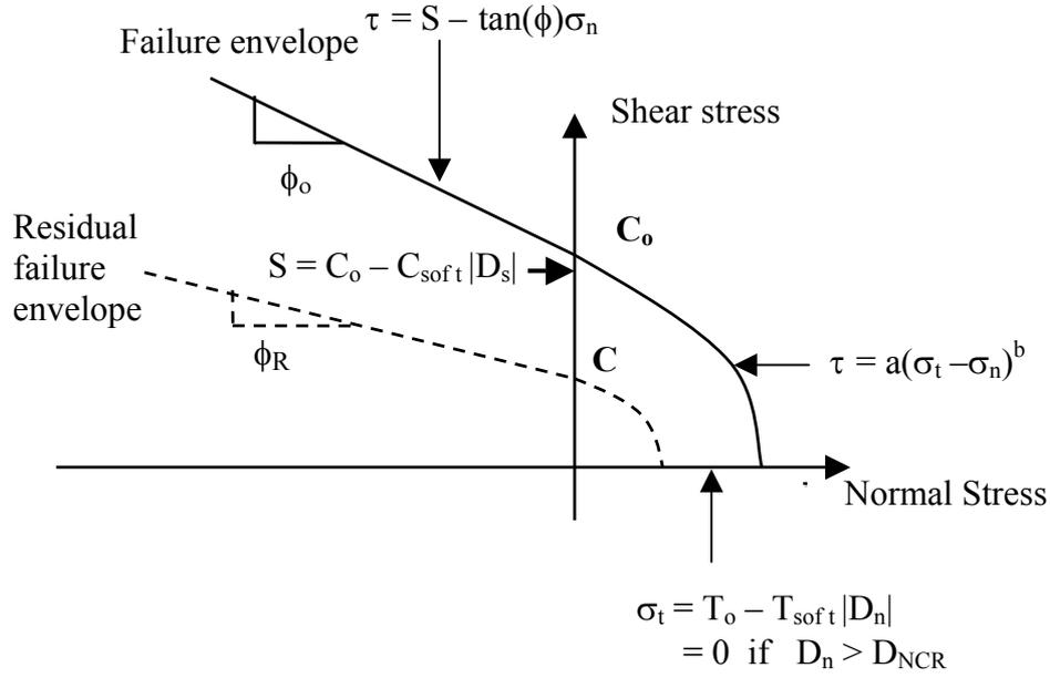
Figure 1. Mohr Coulomb type of failure criterion for determining crack mobilization.
