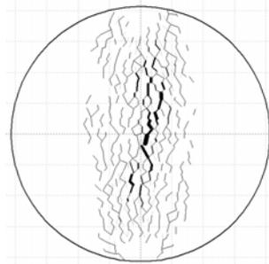
(c) Crack pattern at visible macro-crack
