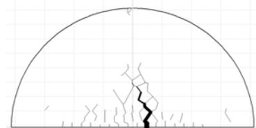
(c) Crack pattern at visible macro-crack
