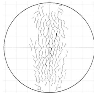
(b) Crack pattern at fracture point
