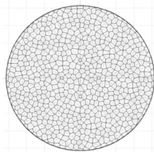
(a) Indirect Tensile Test model
