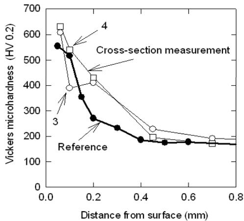
Fig. 2 – Microhardness profiles in the surface layer
