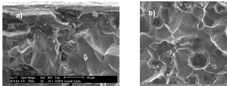
Fig. 4 - Fracture surface of specimen 4 - a) nitrided layer with carbides, b) intercrystalline cleavage in diffusion zone, SEM
