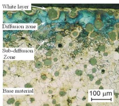
Fig. 1 – Microstructure of the nitrided layer, etched with 5 % molybdenum acid
