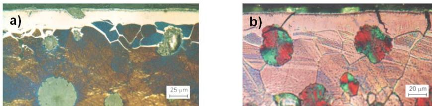
Fig. 7 - Nitrided layer of specimen 4- a) nitrides on the boundaries of ferrite grains, etched with Klemm I [9] b) cracks in white layer, etched with nitric acid, polarized light
