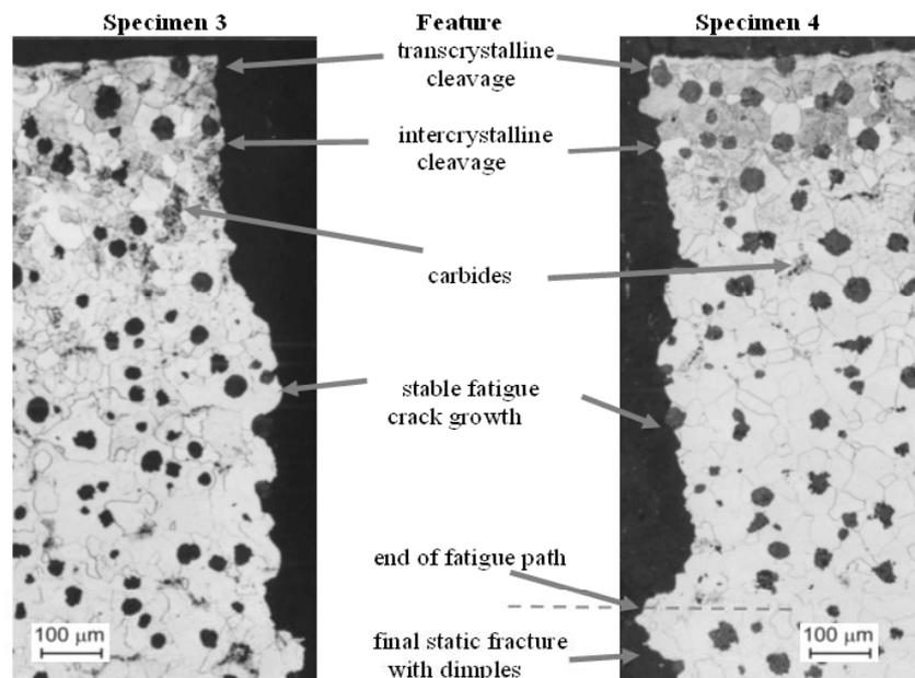
Fig. 6 - Comparison of fatigue crack paths
