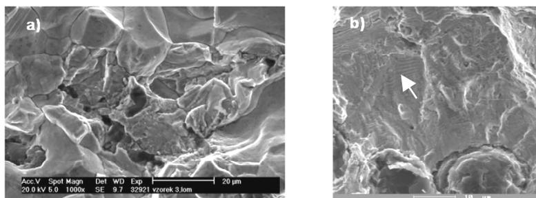
Fig. 5 - Fracture surface of specimen 3 – a) diffusion zone with carbides b) fatigue region with striations, SEM
