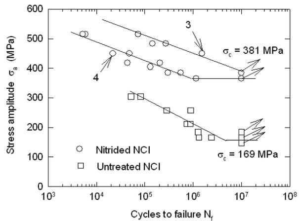
Fig.3 - Fatigue response of NCI in the untreated and nitrided conditions
