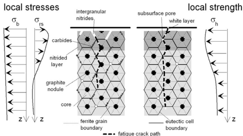
Fig. 8 – Scheme of stress and strength profiles in the nitrided NCI and idealized microstructures and crack paths for short fatigue life (left) and long fatigue life (right)
