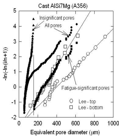
Fig. 3 Extreme value plot of equivalent pore size of an AlSi7Mg
