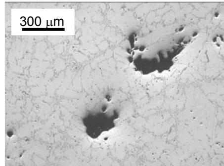
Fig. 2 Examples of shrinkage porosity.
