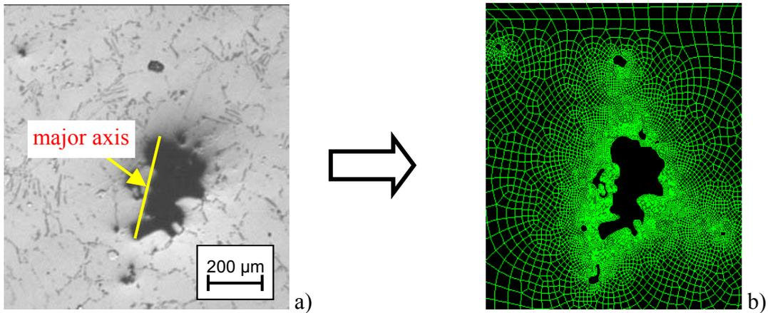
Fig. 5 a) Image of a porosity and b) finite element model of the pore.
