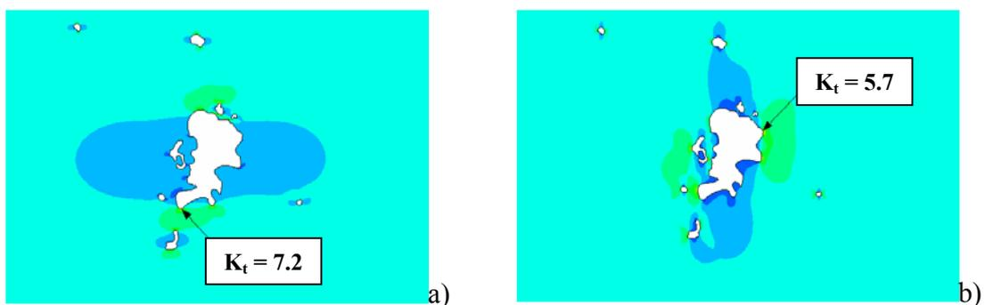
Fig. 6 Theoretical stress concentration at a shrinkage pore
