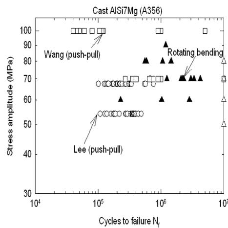
Fig. 4 Comparison of rotating bending fatigue results on cast A356 with push-pull tests results from the literature
