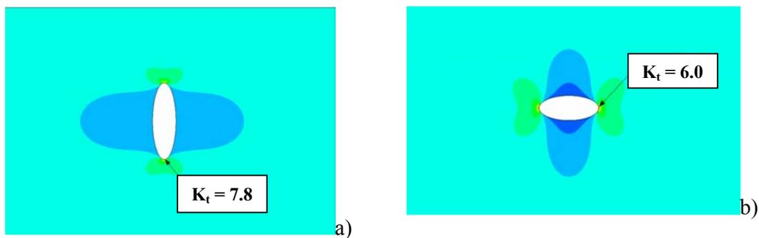
Fig. 8 Theoretical stress concentration at ellipses equivalent to porosity
