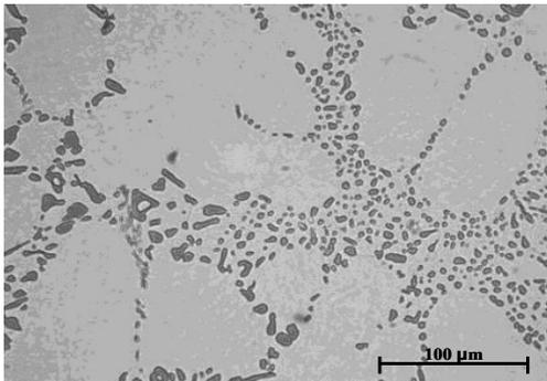
Fig. 1 Microstructure of AlSi7Mg.
