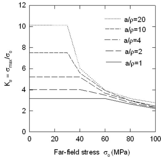
Fig. 9 Evolution of the elastic-plastic stress concentration factor  $K_\sigma$  as a function of the applied far-field load for equivalent ellipses (semi axis/root radius  $a/\rho$ )
