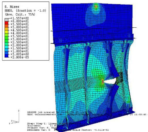
Figure 6 – Mises stress in the damaged panel, crack length 262 mm, for 10000 N load (magnification factor: 561)
