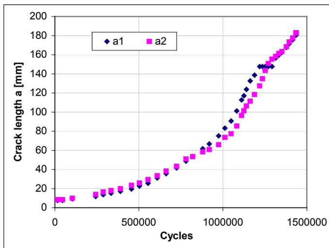
Figure 4. The crack propagation on the two apices
