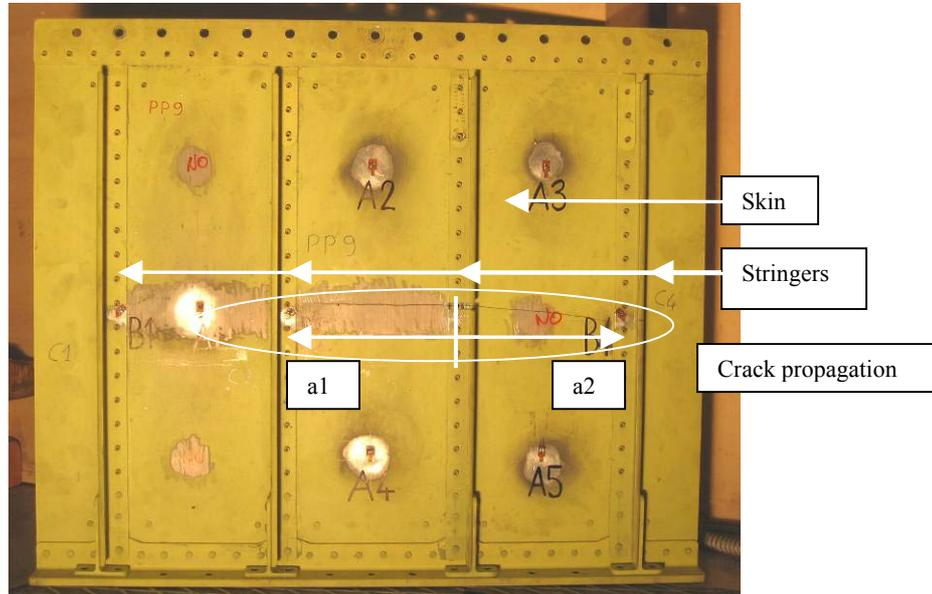
Figure 1. Specimen after the test with crack propagated and strain gauges
