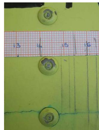
Figure 5. The crack path near the rivet hole
