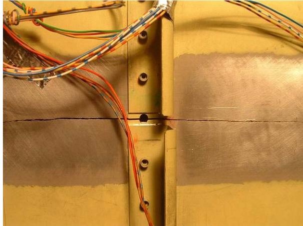
Figure 3. The artificial damage and the crack propagation
