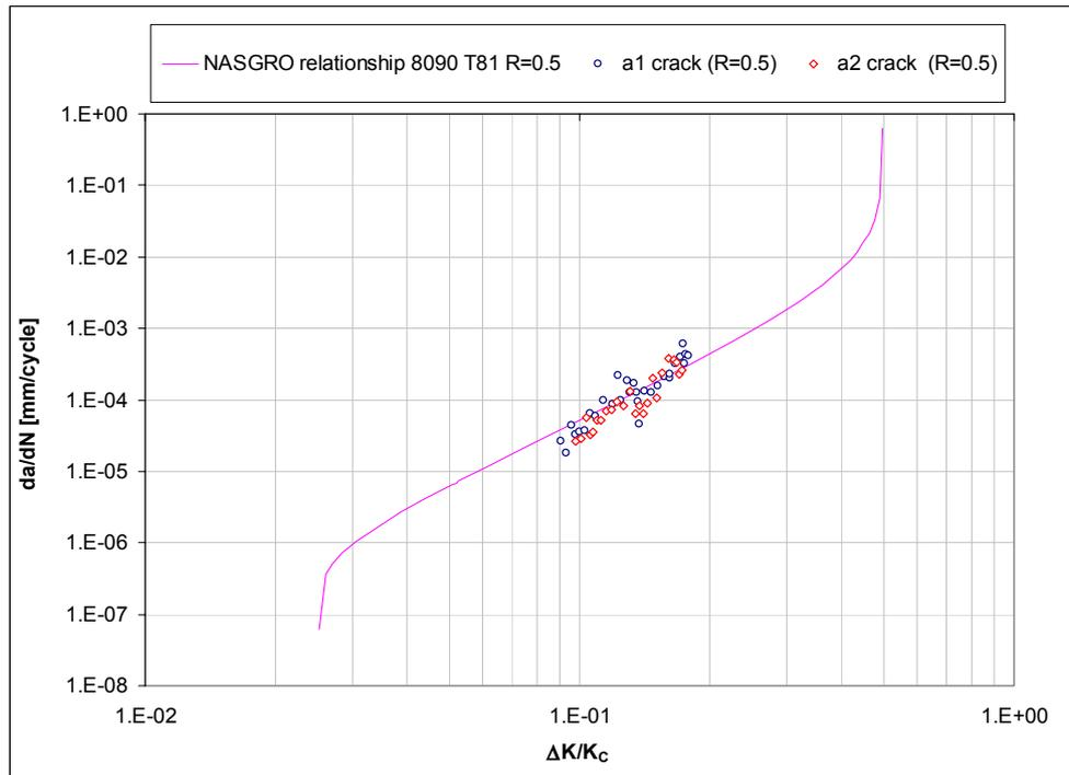
Figure 8 – Comparison between the experimental FEM data with the behavior of the material
