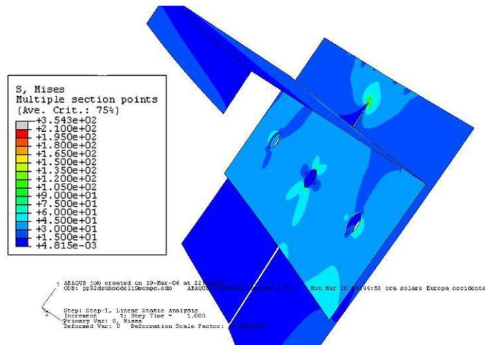
Figure 7 – Mises stress in the damaged panel, submodel, crack 346.5 mm, for 10000 N load (magnification factor: 26)
