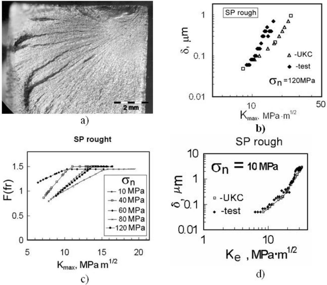
Figure 2. The overview (a) and (b) the striation spacing values, (c) the functional correction  $F(fr)$  against the stress intensity factor  $K_{\text{max}}$  for the different normal stresses, and (d) the striation spacing value against the equivalent of the stress intensity factor  $K_e$  for unpeened and peened specimens and UKC, Eq. 1.
