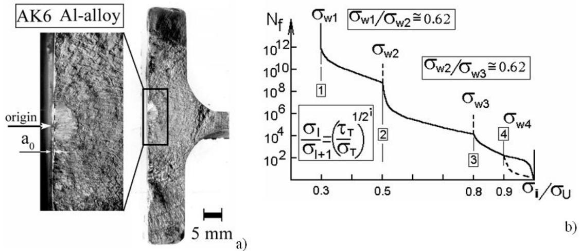
Figure 1. Overview (a) of the fracture surface of the in-service fatigued helicopter longeron in area of  $10^{10}$  cycles because of the fretting damage, and (b) the bifurcation Wöhler diagram: (1-2) VHCF, (2-3) high-cycle-fatigue (HCF), (3-4) low-cycle-fatigue (LCF), and, then, quasi-static fracture. The origin places under the damaged surface in the depth of  $a_0=0.1\text{mm}$ ;  $\tau_T$  and  $\sigma_T$  – theoretical shear and tension material strength.
