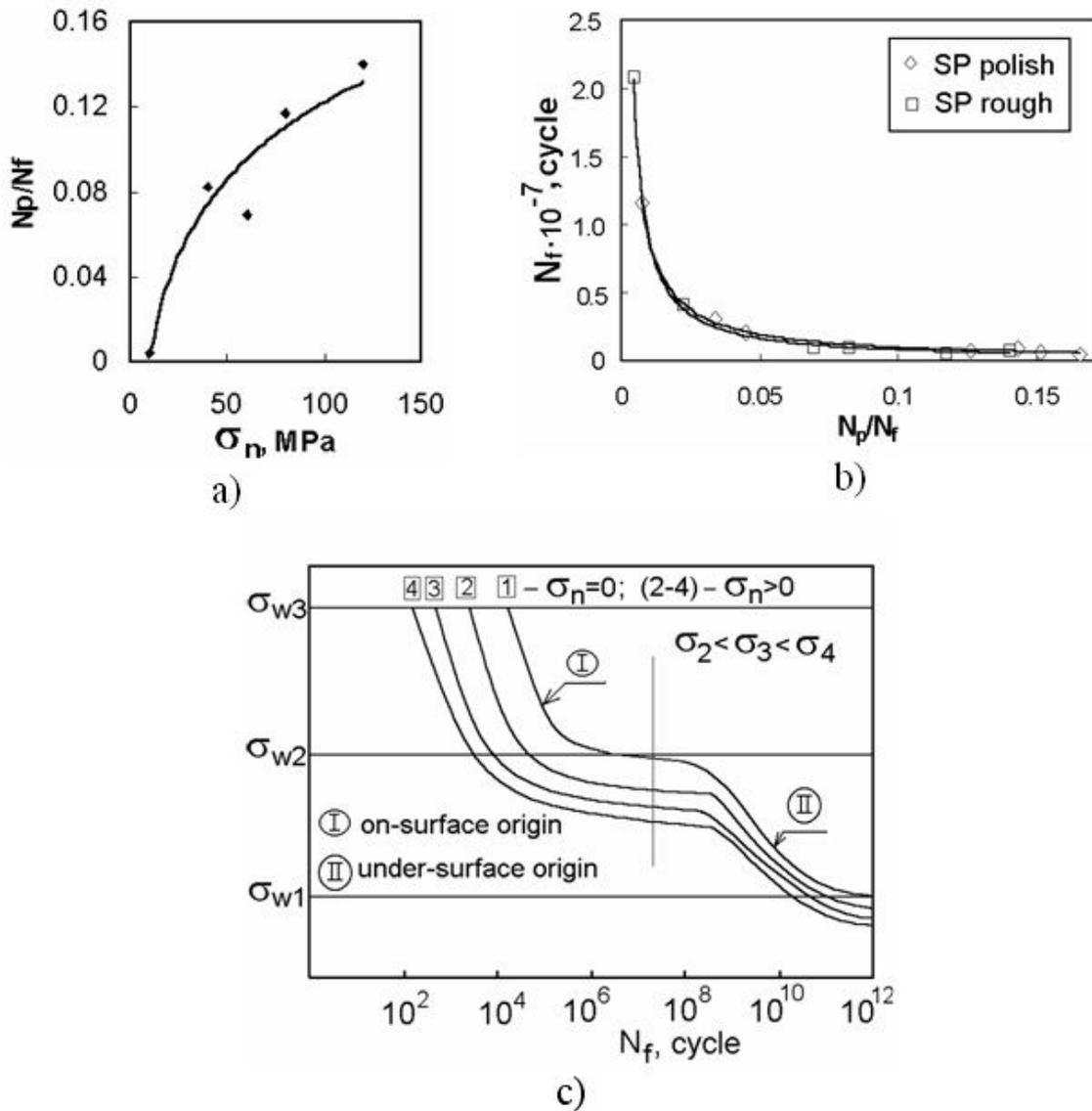
Figure 3. The ratio  $N_p / N_f$  against (a) the normal stress  $\sigma_n$  for “SP polish” specimens, (b) the lifetime to failure  $N_f$  against the ratio  $N_p / N_f$  for “SP polish” and “SP rough” specimens, and (c) the diagram of the  $N_f$ -value dependence on the cyclic loads for various normal stresses,  $\sigma_n$ .
