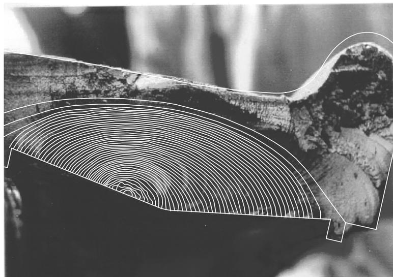
Figure 11. Comparison of simulated crack growth with the real fracture surface of the wheel tyre
