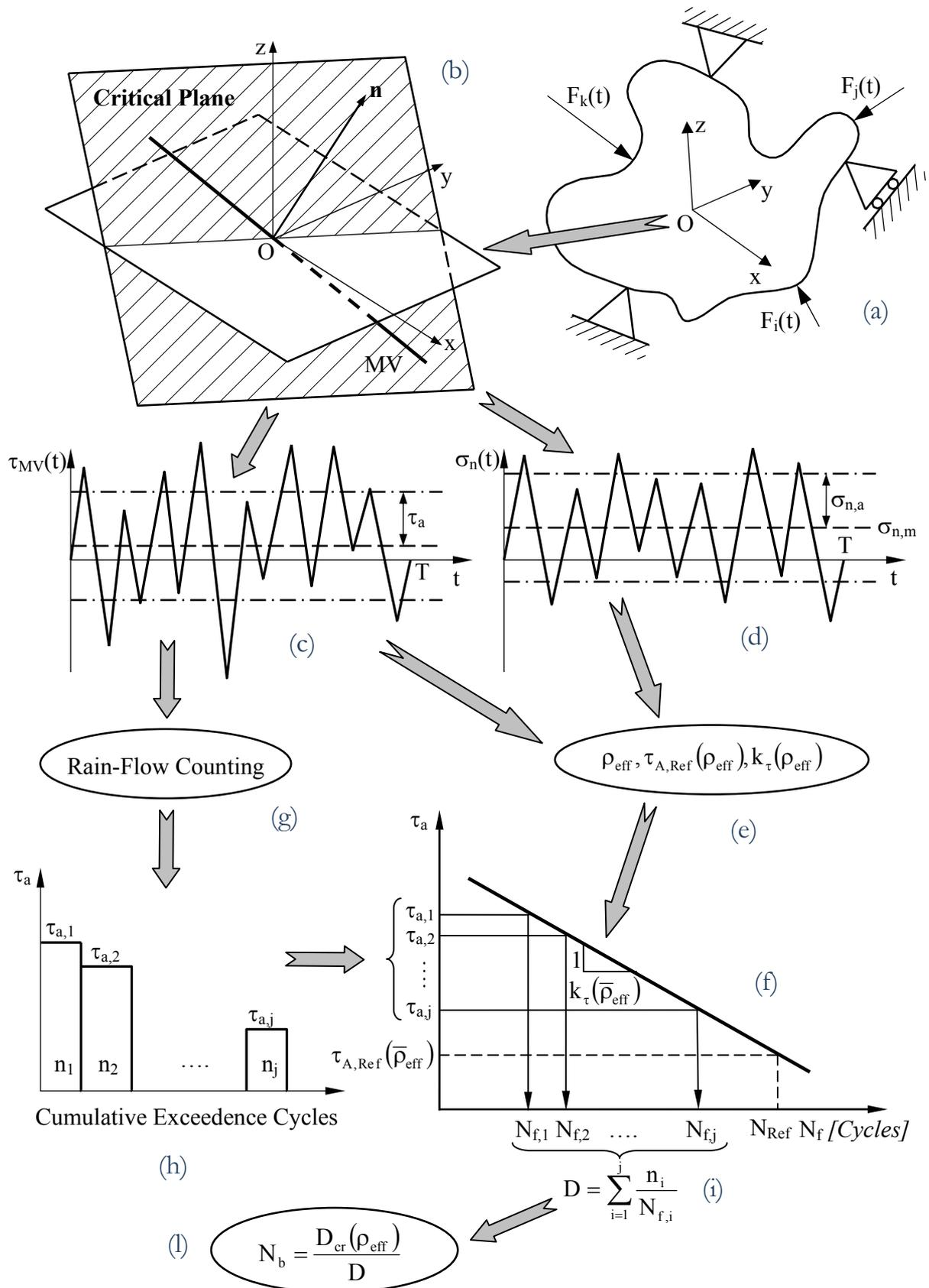
Figure 2: In-field use of the MWCM to perform the fatigue assessment under VA multiaxial fatigue loading.
