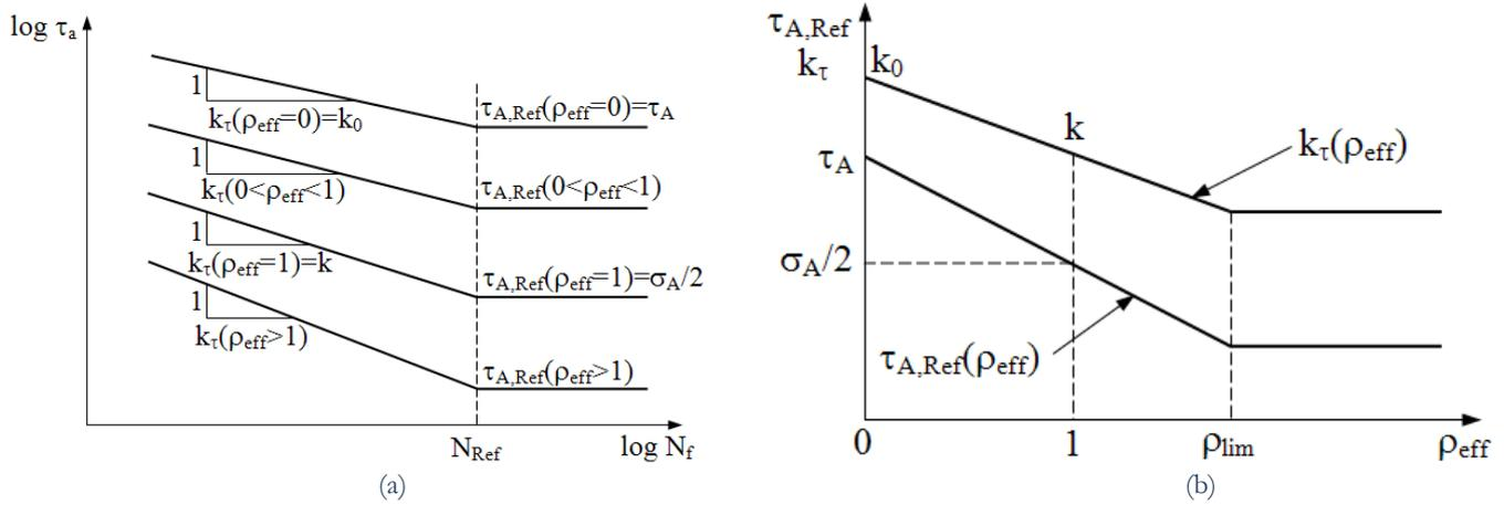
Figure 1: Modified Wöhler diagram (a) and MWCM's governing equations (b).
