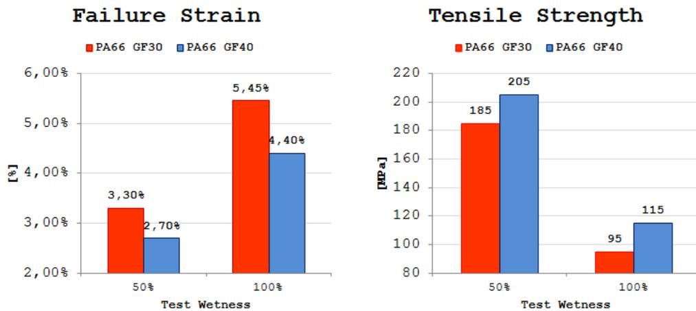
Figure 4: Mechanical characteristics (failure strain, tensile strength) depended on test wetness of PA66 GF30 and PA66 GF40.
