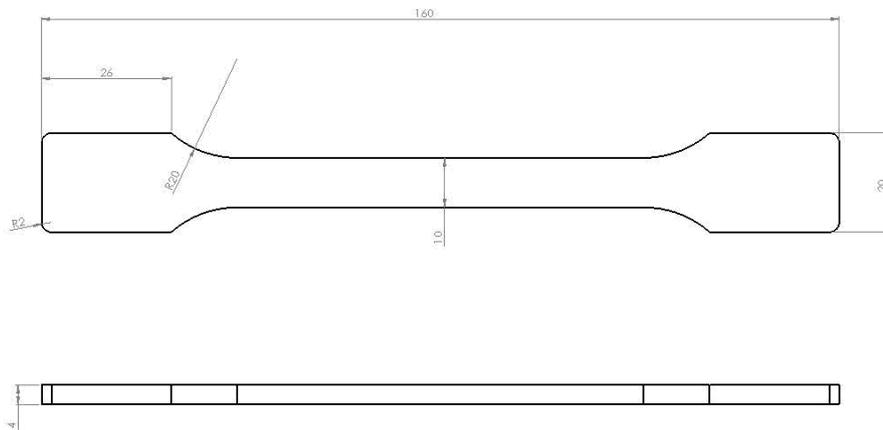
Figure 6: Geometry and dimensions of the specimen [mm].
