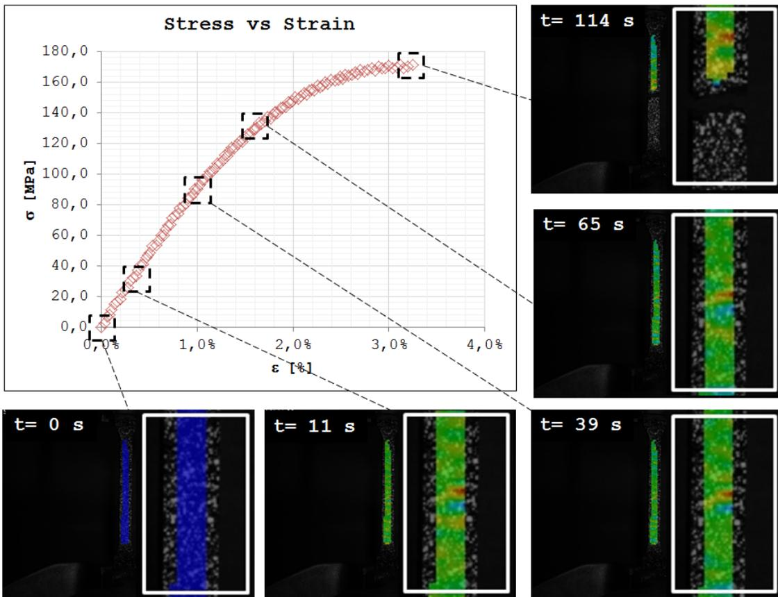
Figure 11: Example given of DIC analysis for tensile test.
