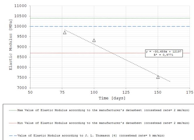
Figure 9: Elastic modulus vs. time.
