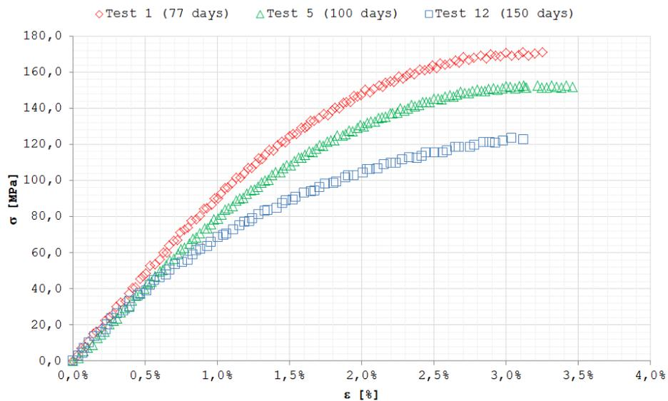
Figure 8: Tensile strength vs strain failure for three different test ( $v = 2 \text{ mm/min}$ ).
