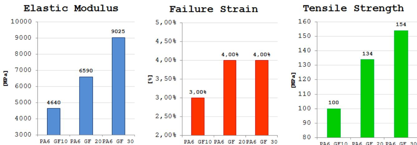
Figure 1: Different mechanical characteristics (elastic modulus, failure strain, tensile strength) depended on wt% of fiber (PA6 GF10, PA6 GF 20, PA6 GF30).
