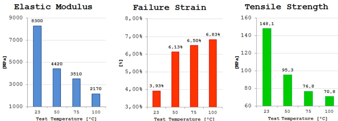
Figure 3: Mechanical characteristics (elastic modulus, failure strain, tensile strength) depended on test temperature of PA66 GF33.
