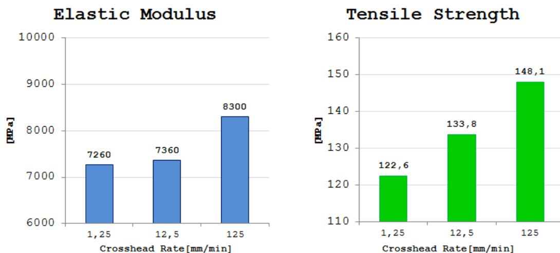
Figure 2: Different mechanical characteristics (elastic modulus, tensile strength) depended on crosshead rate of PA66 GF33.
