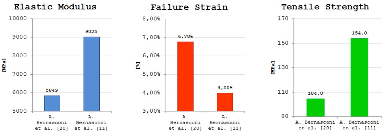
Figure 5: Mechanical characteristics (elastic modulus, failure strain, tensile strength) for PA6 GF30.
