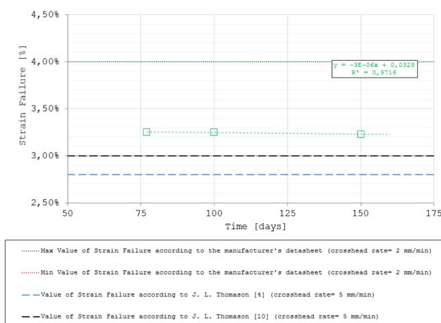
Figure 10: Strain failure vs. time.
