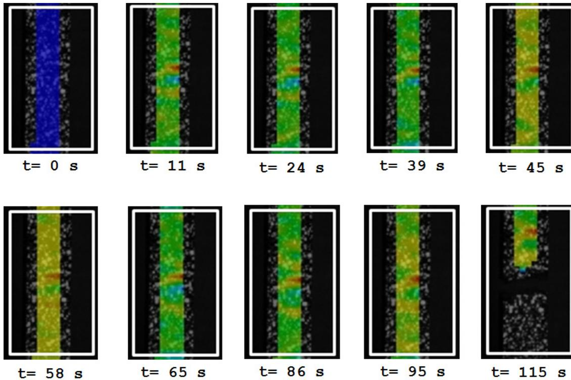
Figure 12: Detail DIC images at progressive time test for tensile test (Fig. 11).
