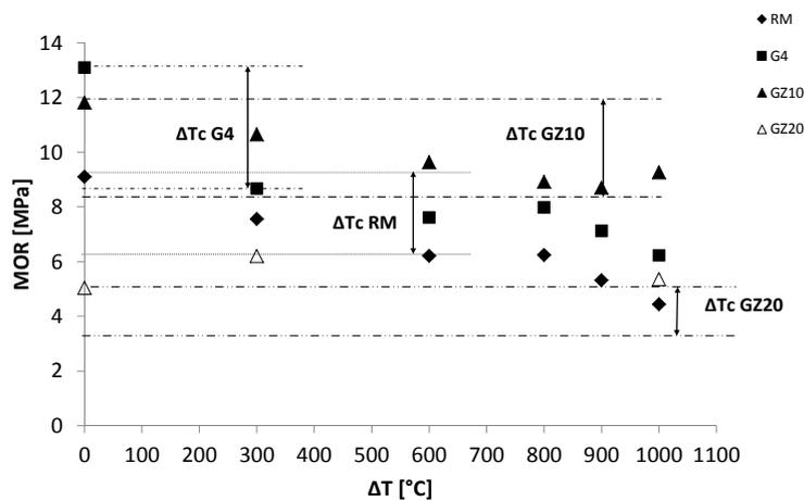
Figure 4: Residual MOR mean values determined on RM, G4, GZ10 and GZ20 after water quenching and their corresponding critical quenching temperature ( $\Delta T_c$ ).
