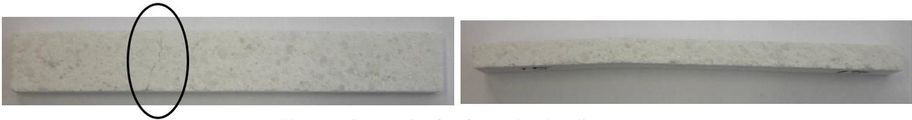
Figure 2: G4 sample after four points bending test.
