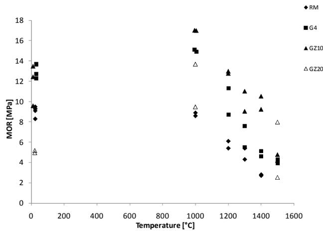
Figure 3: MOR values determined by the four-point flexural tests carried out on RM, G4, GZ10 and GZ20.
