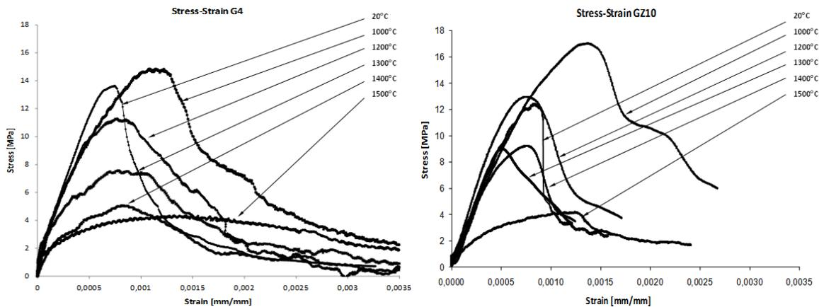
Figure 1: Stress-strain curves for the evaluation of thermomechanical properties of the refractory mixture G4 (left) and GZ10 (right).
