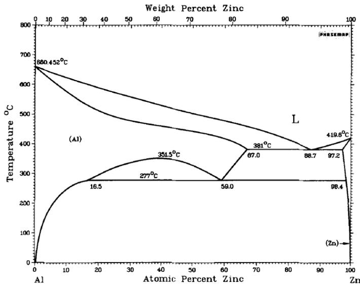
Figure 1: Al-Zn Phase Diagram.
