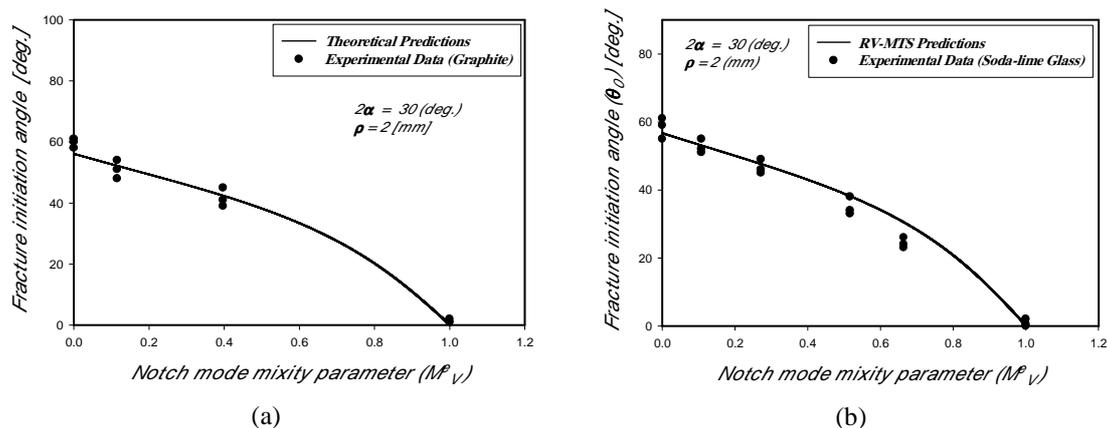
Fig. 5. Curves of mixed mode fracture initiation angles for V-notches in (a) graphite and (b) soda-lime glass, with notch opening angle of  $30^\circ$  and notch tip radius of 2 mm.
