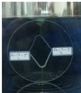
Fig. 3. The V-BD soda-lime glass specimen in a mixed mode I/II fracture test.
