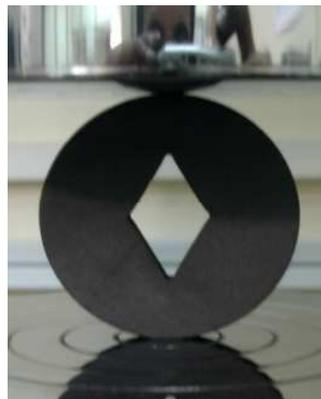
Fig. 2. The V-BD graphite specimen in a mode I fracture test.
