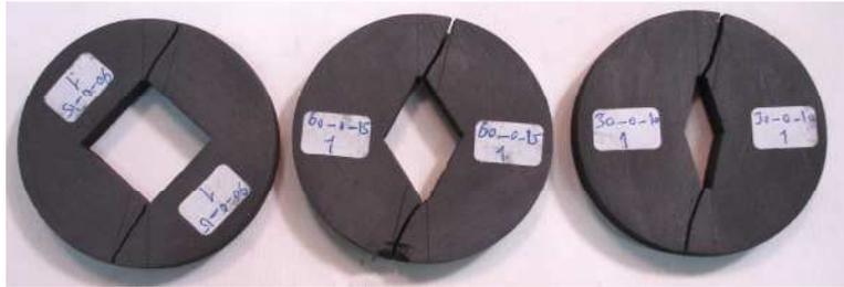
Fig. 4. The graphite specimens broken after mixed mode I/II fracture tests.
