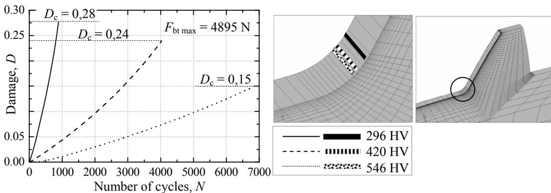
Figure 3. Maximum tooth root damage accumulation, 42 CrMo 4
