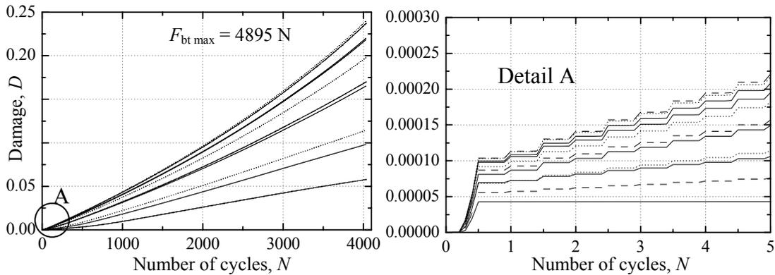
Figure 2. Tooth root damage accumulation, 42 CrMo 4 – 420 HV
