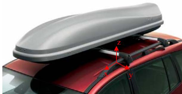
Figure 1: Multiaxial loading of the roof bar.
