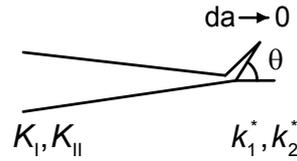
Figure 5. Crack tip deflection.
