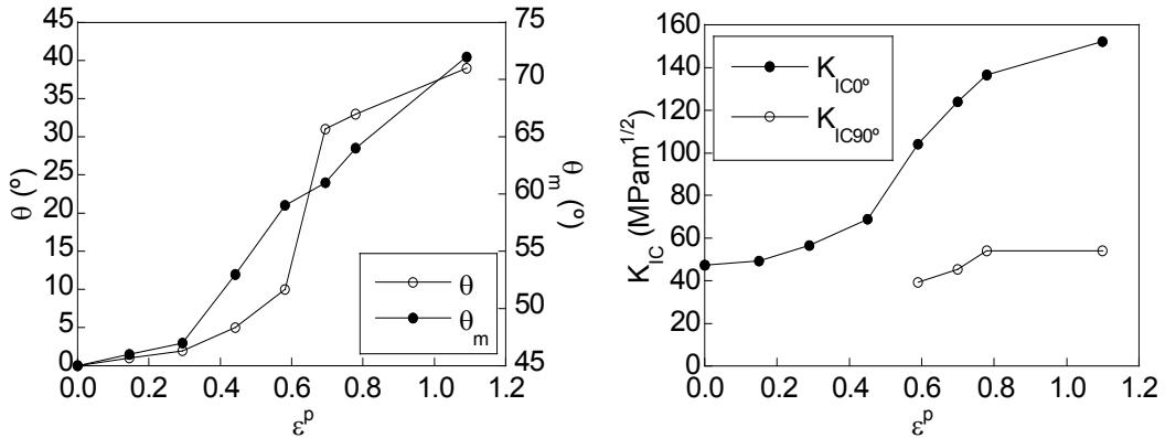
Figure 9. Fracture angle (left) and fracture toughness  $K_{IC0^\circ}$  and  $K_{IC90^\circ}$  (right).
