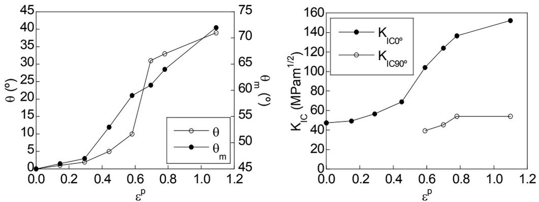
Figure 9. Fracture angle (left) and fracture toughness  $K_{IC0}$  and  $K_{IC90}$  (right).
