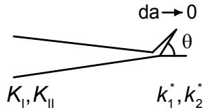
Figure 5. Crack tip deflection.
