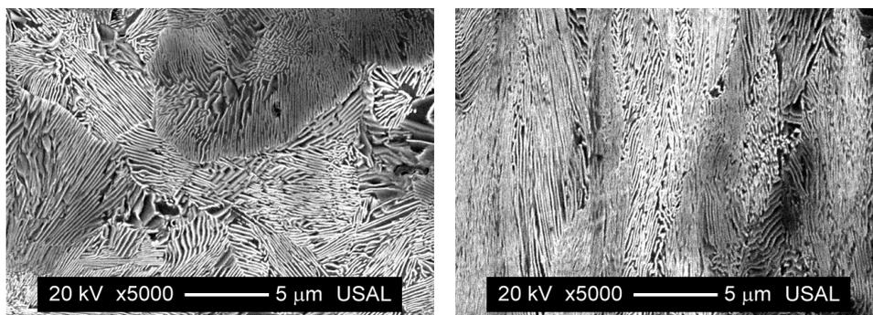
Figure 1. Microstructure, longitudinal section, B0 (left) and B7 (right).
