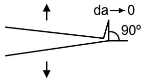
Figure 6. Crack tip deflection towards  $90^\circ$ .
