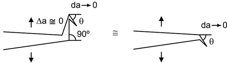
Figure 7. Crack tip deflection towards  $\theta$ .
