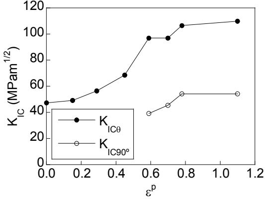
Figure 8. Fracture toughness,  $K_{IC0}$  and  $K_{IC90^\circ}$ .
