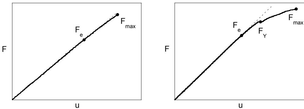
Figure 4. Load-displacement curve, B0 (left) and B7 (right).
