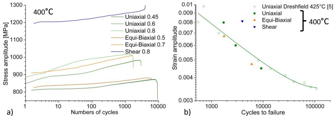
Figure 5: a) Cyclic deformation curves of the different uniaxial and biaxial tests. b) Lifetimes for all performed tests compared to data of the literature.
