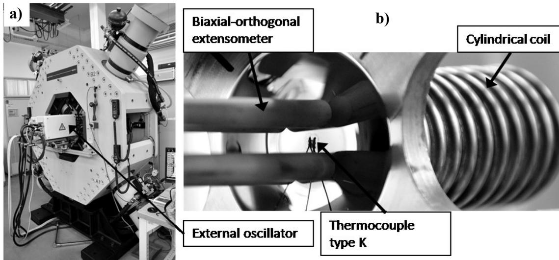
Figure 2: a) Biaxial-planar tension-compression machine with external oscillator and cylindrical coil. b) Applied extensometer and thermocouple as well as the aligned cylindrical induction coil on the back side of the cruciform specimen.
