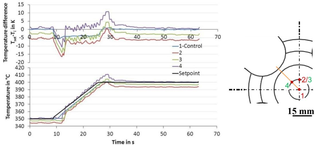
Figure 4: Sample behavior of the cruciform specimen for a temperature ramp signal demonstrated by 4 thermocouples, which are placed in the gauge area.
