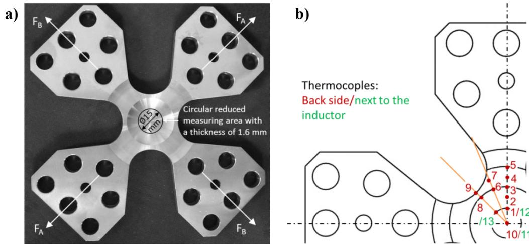
Figure 3: a) Specimen geometry and b) position of the thermocouples attached by welding.
