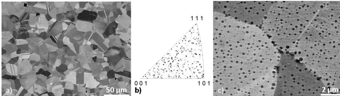
Figure 1: a) SEM image of the microstructure, b) inverse pole figure, which shows no preferred grain orientation, c) SEM image of the monomodal distribution of spherical  $\gamma'$ -precipitates.
