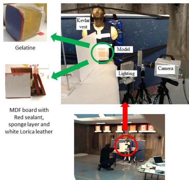
Figure 1. Experimental setup: the physical model was placed on a Kevlar vest with halogen lighting and recorder using a high speed camera.
