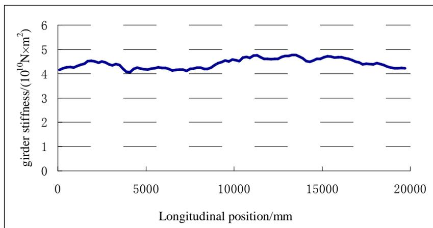
Figure 6.stiffness distribution curve
