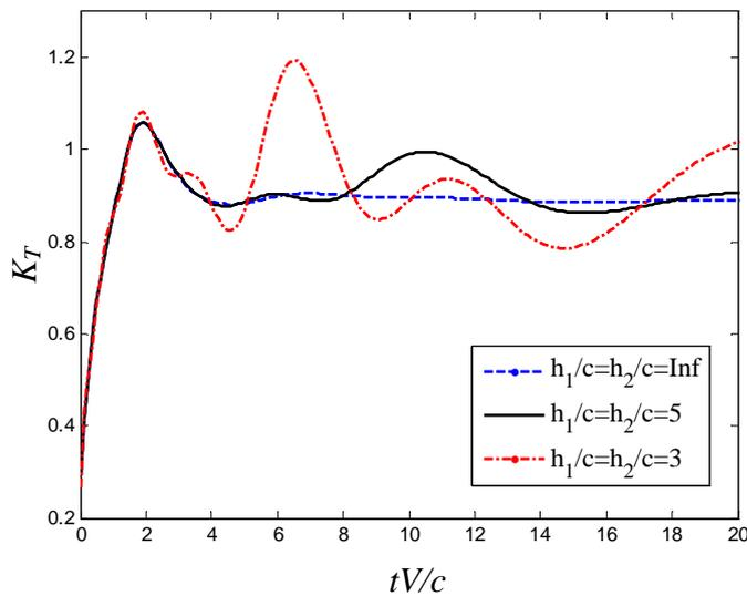
Figure 3. Normalized dynamic SIFs  $K_T$  vs normalized time for different geometric size  $h_1/c = h_2/c$  when  $\beta = +1$ ,  $V = V_e$
