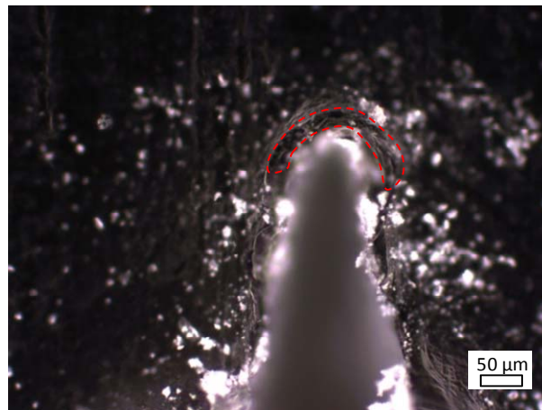
Figure 7. Crack tip front of a specimen with a notch introduced via razor sliding where some damage can be observed ahead of the crack front (initial crack tip radius of 35 \mu\text{m} )
