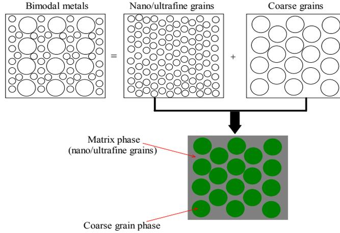
Fig. 1 Schematic drawings of bimodal grain size distributions in polycrystalline materials with assumption of the composite mixture model.
