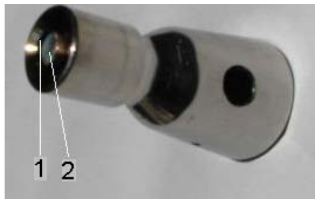
Fig. 5. Appearance of removable cathode assembly with explosive emission: 1 – ring cylindrical cathode; 2 – sample.
