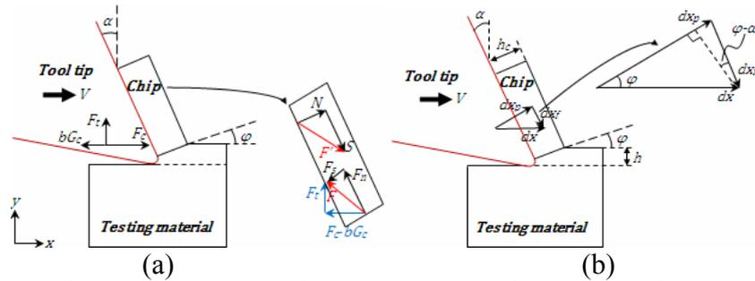
Figure 1. Schematic diagrams of orthogonal cutting (a) force relationship of the cutting system and (b) geometrical relationship of displacements of forces during cutting.
