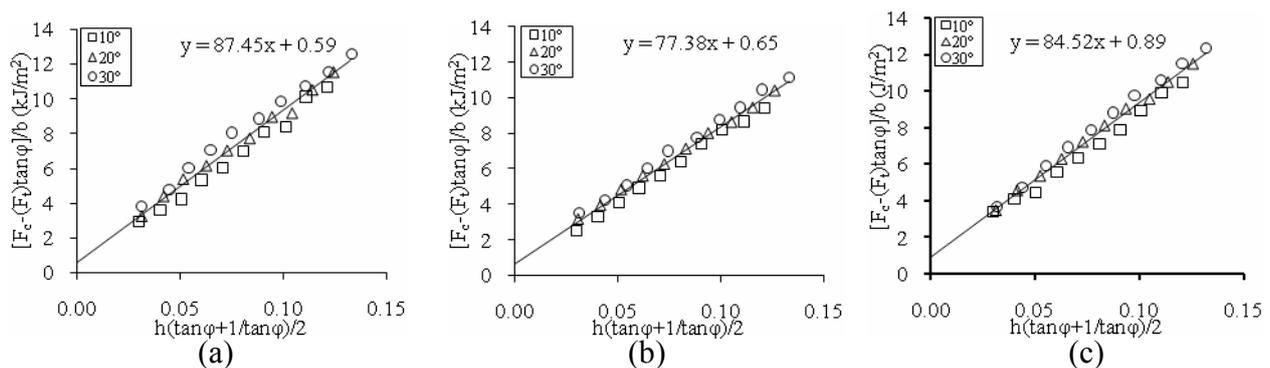
Figure 2. Cutting results for (a) pure epoxy with specimen width  $b=5.57mm$ , (b) 10% nano-rubber epoxy with specimen width  $b=5.04mm$ , and (c) 10% nano-silica epoxy with specimen width  $b=5.40mm$ . The cutting velocity was at 1 mm/s. The legend shows the rake angle in degrees.
