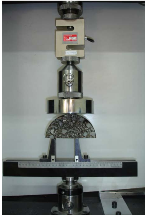
Figure 2. Three point test set-up
