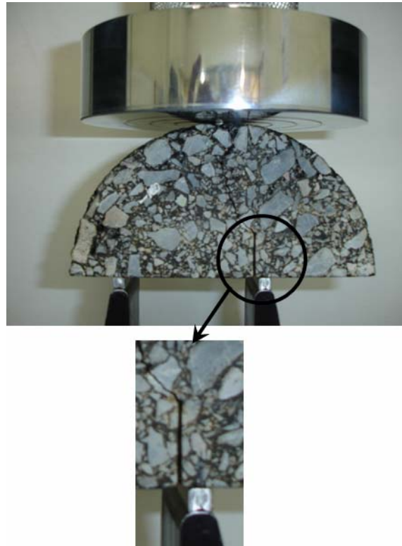
Figure 6. Fracture test using second set-up
