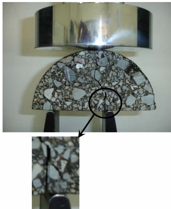
Figure 3. Fracture test using first set-up
