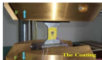
Figure 4b The picture of coupon testing
