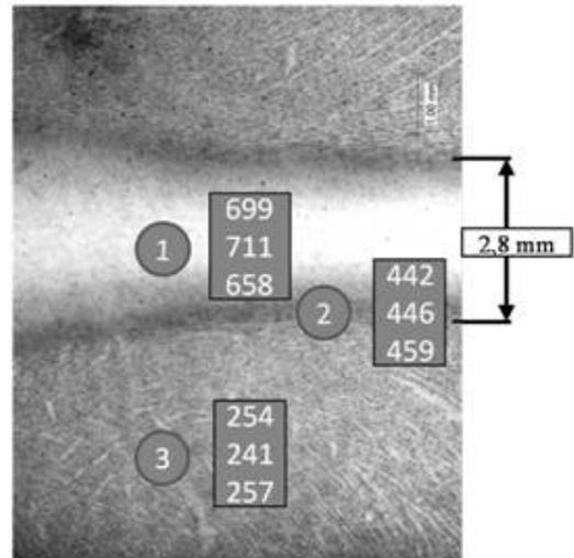
Figure 3. Vickers hardness of the different phases
