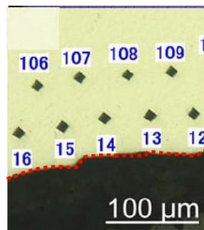
Figure 13. Micro-hardness indentations along section of crack face (dotted red line)
