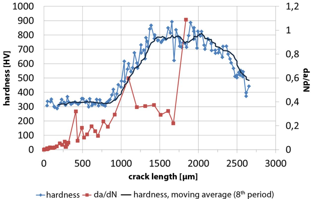
Figure 12. Microstructure dependent growth rate of crack #1
