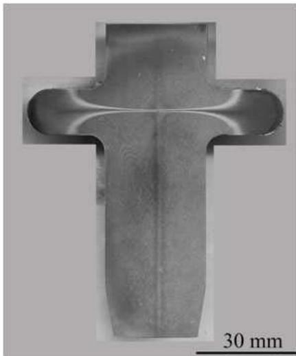
Figure 2. Micrograph of the flange shaft, etched
