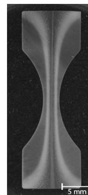
Figure 8. Microspecimen, etched
