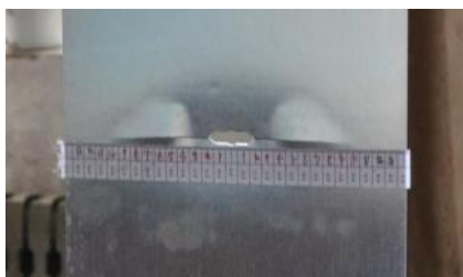
Fig 1 Delamination shape in FML during testing
