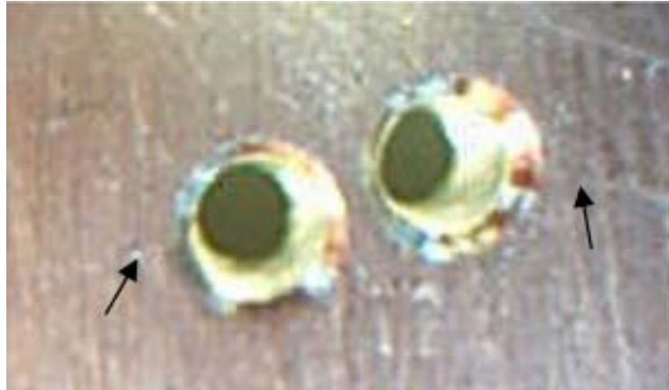
Fig.6, the first crack initiates from the outer edge of the hole
