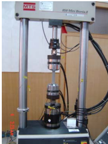
Fig.2, The fatigue test using MTS
