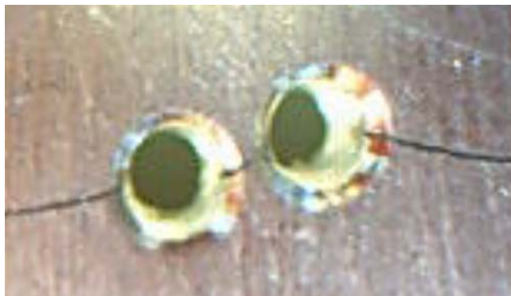
Fig.8, the first crack initiates from the outer edge of the hole
