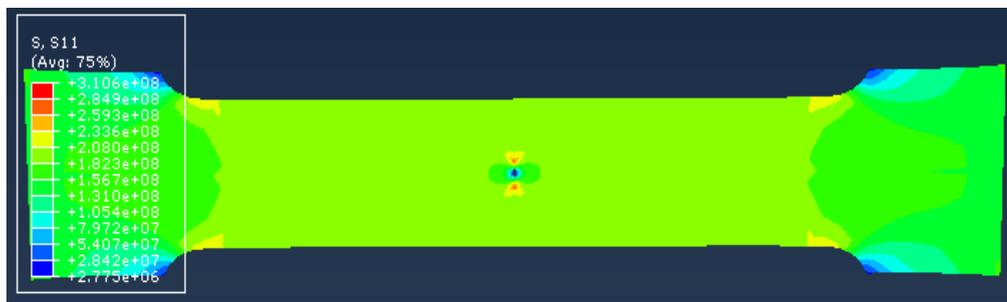
Figure 3. Component  $\sigma_{xx}$  (in the tension direction) of the stress tensor
