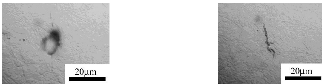
Figure 7. Cracks observed in Steel C in low (RH25%, left) and high (RH85%, right) humidity, respectively (Axial stresses applied in the horizontal direction)
