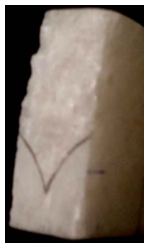
Figure 6. Fracture surface of CCNSCB specimen
