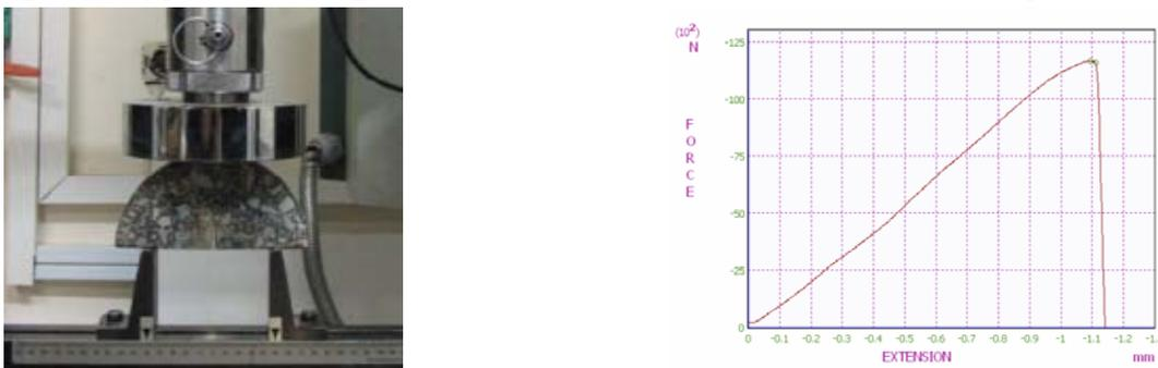
Figure 3. loading setup used for testing of SCB specimen made of asphalt mixture and a typical load-displacement curve obtained for  $-15^{\circ}\text{C}$ .
