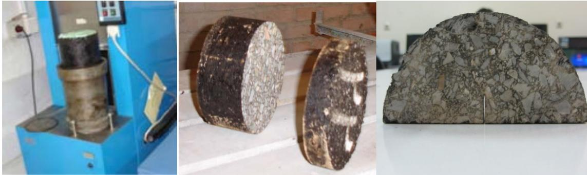
Figure 2. Some of the steps for preparing the SCB test specimens.
