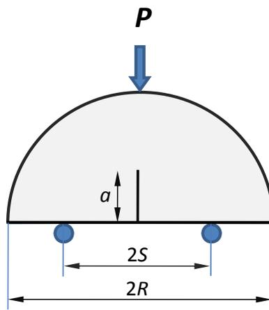
Figure 1. The edge cracked SCB specimen subjected to symmetric bend loading.
