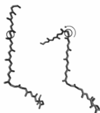
Figure 2. Pivot polypeptide chain by changing torsion angles
