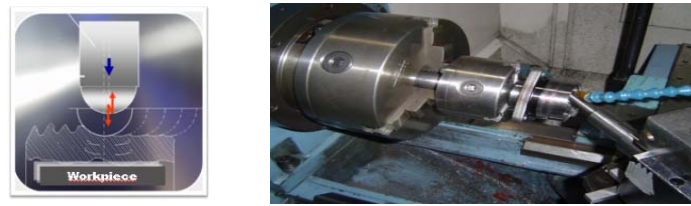
Figure 1. UNSM Mechanism and UNSM Device with CNC Lathe for Hub Bearings
