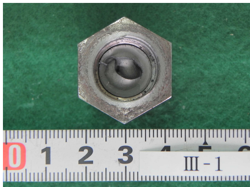
(c) \alpha=\alpha_{\text{middle}} (fatigue life 184,770 cycles)
