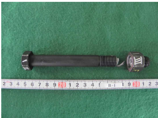
(c) \alpha=\alpha_{\text{middle}} (fatigue life 184,770 cycles)
