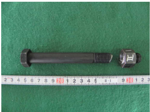
(b) \alpha=\alpha_{\text{small}} (fatigue life 242,810 cycles)
