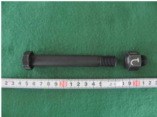
(a) \alpha=0 (fatigue life 151,860 cycles)
