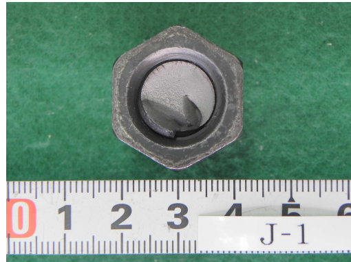
(a) \alpha=0 (fatigue life 151,860 cycles)
