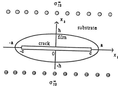
Fig. 1. Schematic illustration of a thin-film-covered Mode III crack under external applied loads in the z plane.
