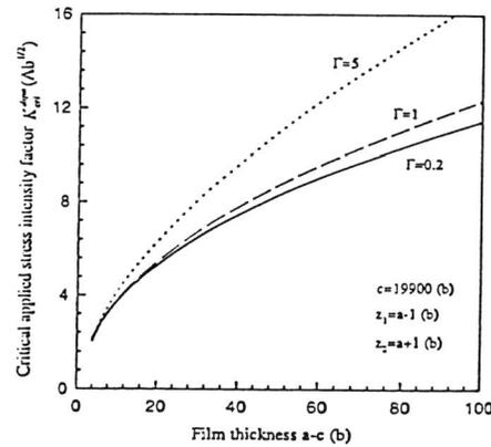
Fig. 6. The critical applied stress intensity factor needed to emit a dislocation dipole with the core size of  $2b$  from the interface increases with increasing the film thickness.
