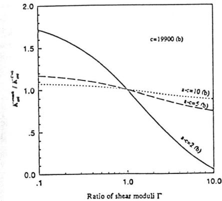
Fig. 3. The normalized critical applied stress intensity factor  $K_{crit}^{crack} / K_{crit}^{\Gamma=1}$  for dislocation emission from the crack tip as a function of the shear modulus ratio for the film thickness  $a-c=2b, 5b$  and  $10b$ .
