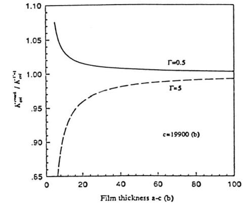
Fig. 4. The normalized critical applied stress intensity factor  $K_{crit}^{crack} / K_{crit}^{\Gamma=1}$  for dislocation emission from the crack tip as a function of the film thickness for  $\Gamma=0.5$  and  $\Gamma=5$ .
