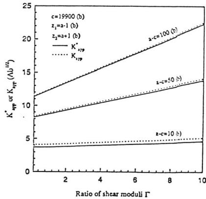
Fig. 5. The critical applied stress intensity factors needed to emit dislocations in the film and substrate at  $1b$  away from the interface are proportional to the ratio of shear moduli.
