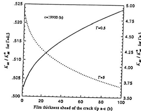
Fig. 2. The normalized stress intensity factors of  $K_{III} / K_{III}^0$  as a function of the film thickness for  $\Gamma=0.5$  and  $\Gamma=5$ .
