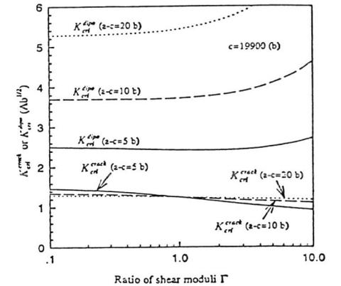
Fig. 7. Comparison of the critical applied stress intensity factors  $K_{cri}^{crack}$  and  $K_{cri}^{dipo}$  needed respectively to emit a dislocation from the crack tip and to emit a dislocation dipole from the interface.
