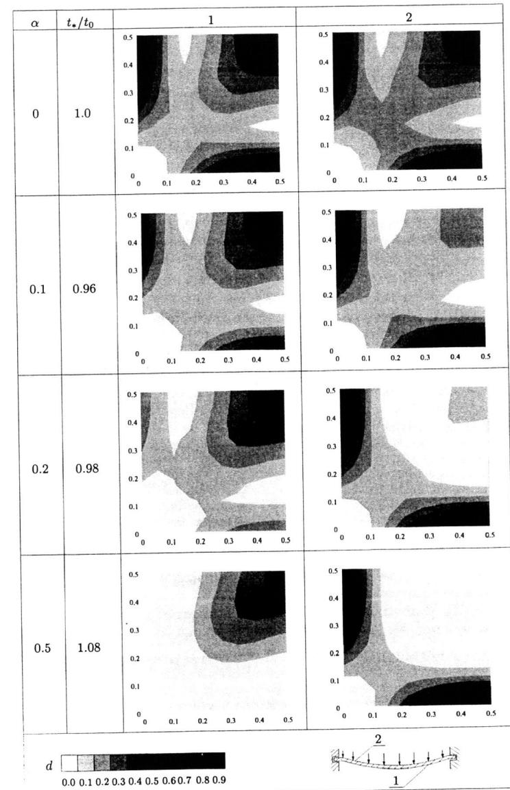
Fig. 2 Distribution of the damage variable on two plate sides,  $t_0$  is the failure time in the case  $\alpha = 0$
