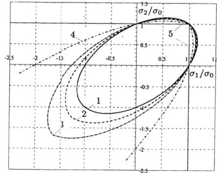
Fig. 1 Isochronous rupture surfaces: 1 -  $\alpha = 0$ ; 2 -  $\alpha = 0.1$ ; 3 -  $\alpha = 0.2$ ; 4 -  $\alpha = 0.5$ ; 5 -  $\alpha = 1$
