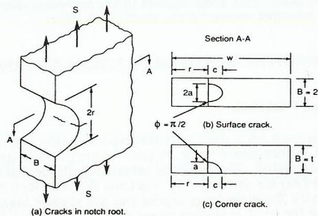
Fig. 1 SENT specimen for fatigue and small-crack test.
