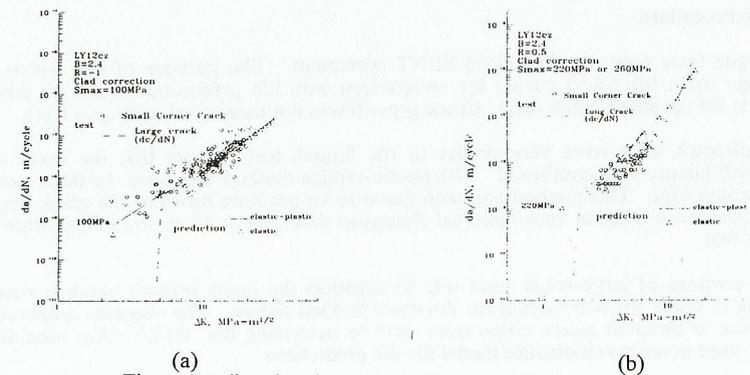
Fig. 4 Predicted and experimental small-crack growth rates.
