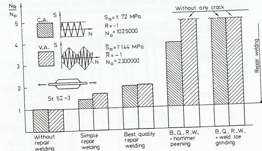
Fig.2 Comparison of remaining fatigue lives by different repair welding procedures
