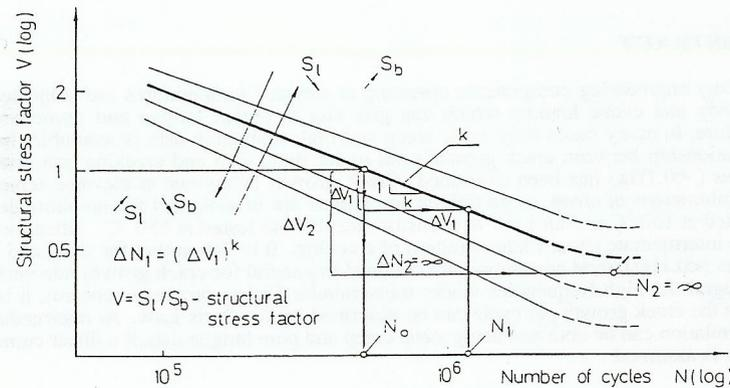
Fig.4 Structural stress factor and extended fatigue lives
