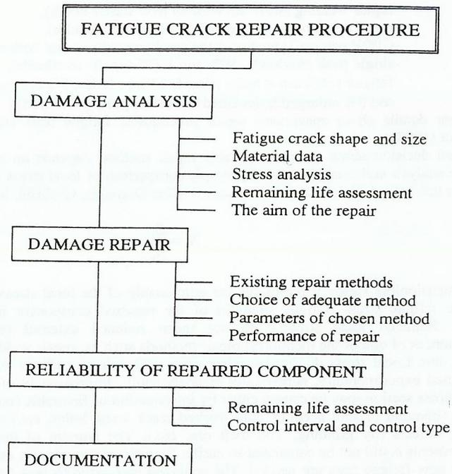
Figure 1 The suggested fatigue crack repair procedure
