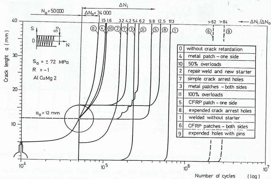
Fig.3 Comparison of remaining fatigue lives by different crack repair procedures
