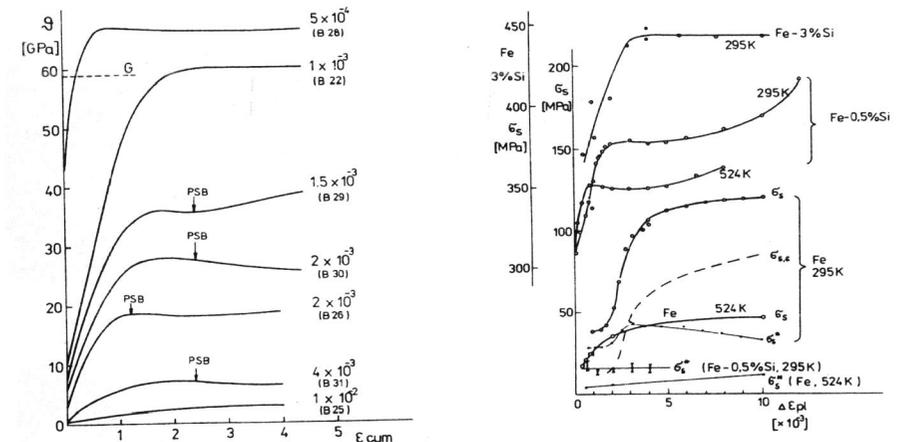
Fig. 2 Cyclic hardening curves for Fe-0.5%Si, 295 K. The arrows indicate formation of PSB's.
