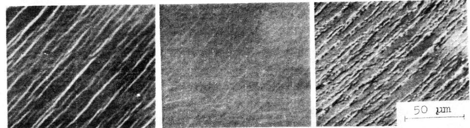
Fig. 4 Slip line pattern on the top face of Fe-0.5%Si single crystal,  $\Delta \epsilon_{pl} = 0.0015$ , 295 K. The surface was repolished after 1600 cycles. The same place on the surface. a) additional 1/2 cycle b) 1 cycle c) 675 cycles
