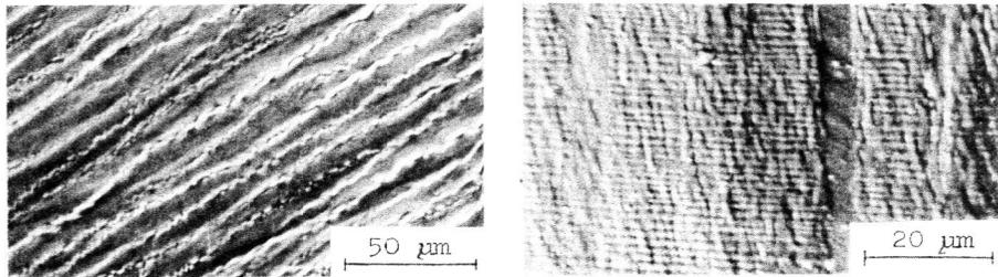
Fig. 5 Slip line structure in PSB's.
